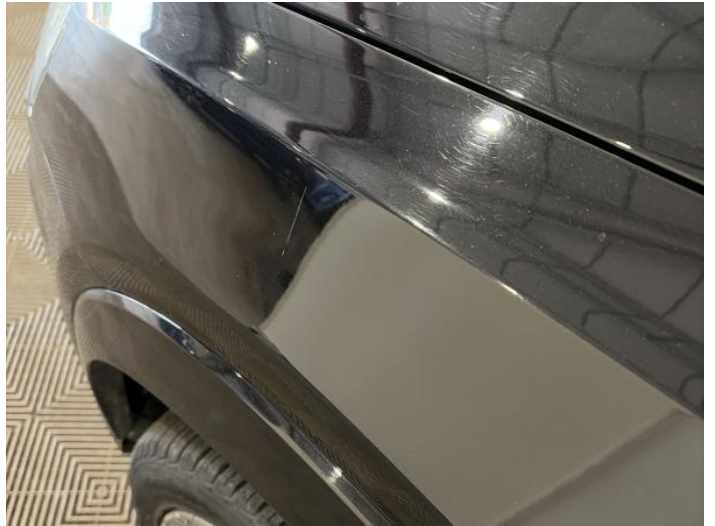
4: Wing nsf Scratched Over 25mm Thru Paint
