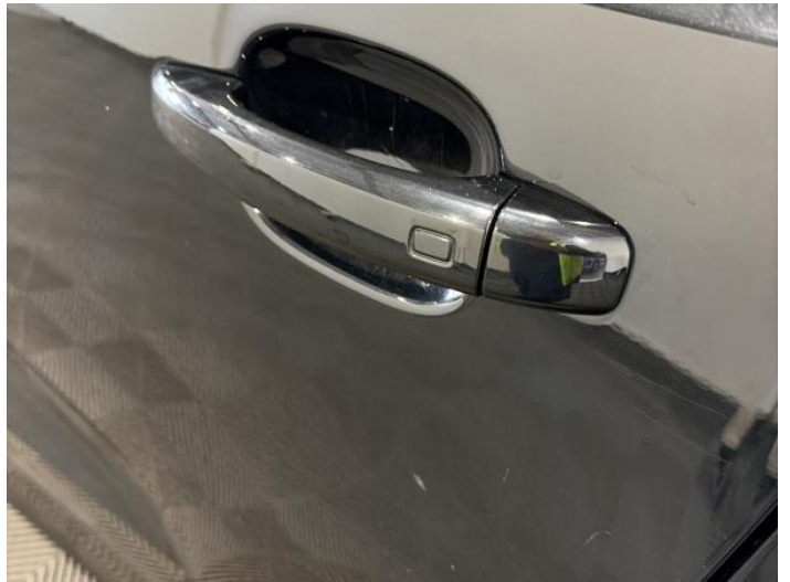
6: Door nsr Scratched Over 25mm Thru Paint
