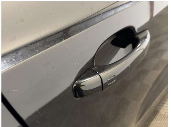
12: Door osr Scratched UpTo 25mm Thru Paint
