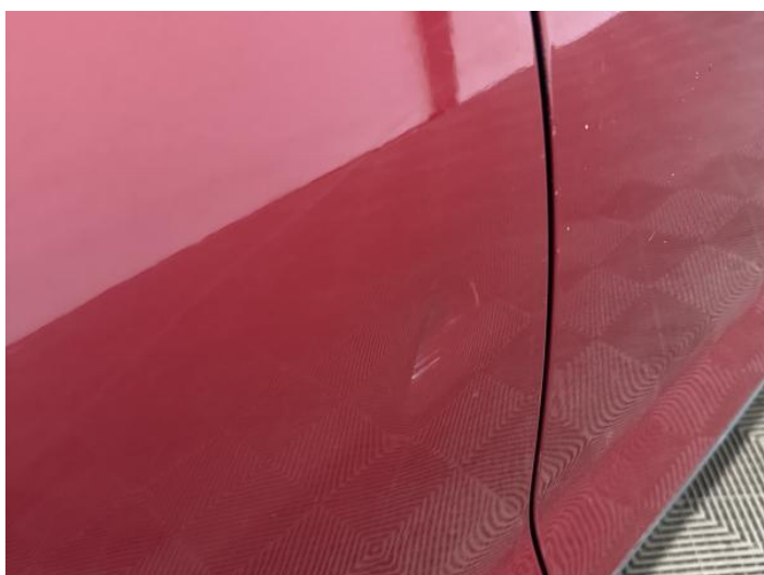
11: Door osr Dented With Paint Damage
