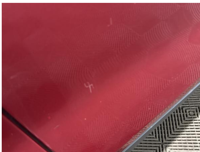
12: Door osf Scratched UpTo 25mm Thru Paint
