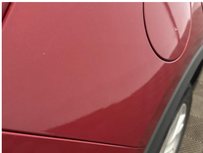
10: Qtr Panel osr Dented With Paint Damage
