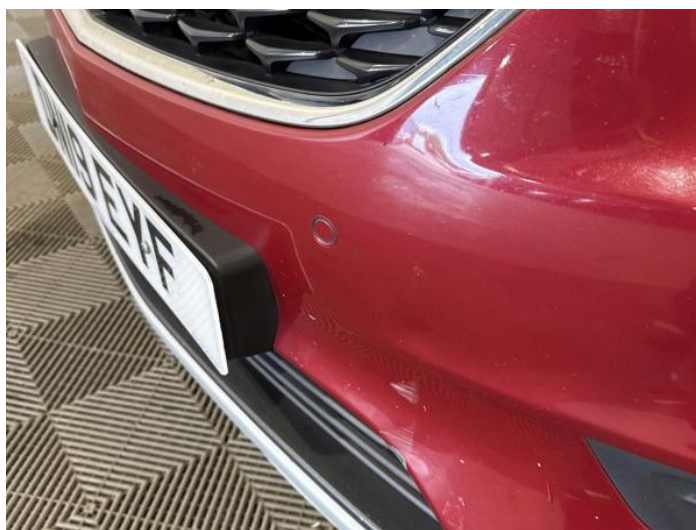
2: Bumper Front Poor Previous Repair Poor Paint
