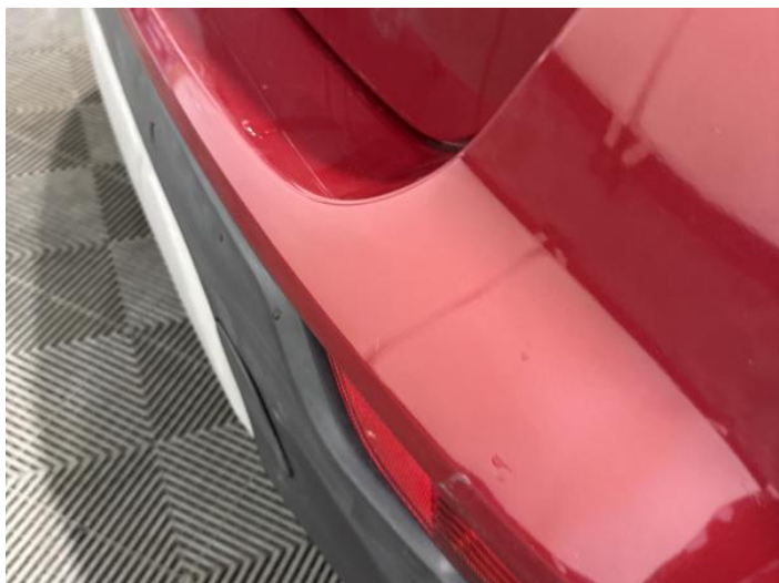
9: Bumper Rear Scratched 25 to 100mm Thru Paint
