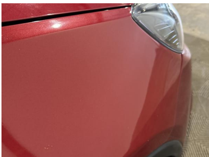
13: Wing osf Poor Previous Repair Rippled UpTo 30%
