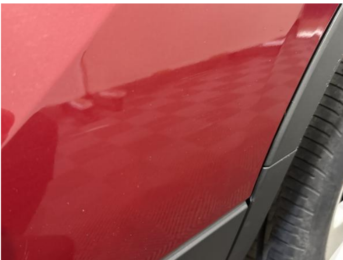
7: Door nsr Scratched Over 25mm Thru Paint
