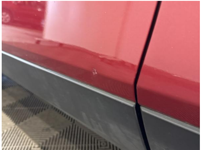
6: Door nsf Scratched Over 25mm Thru Paint
