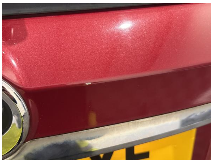
14: Tailgate Poor Previous Repair Poor Paint
