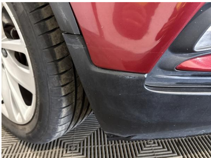
15: Bumper Front Moulding Broken Replace
