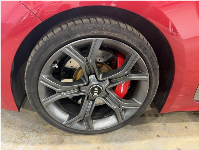
15: Wheel nsf Scratched Up To 50mm
