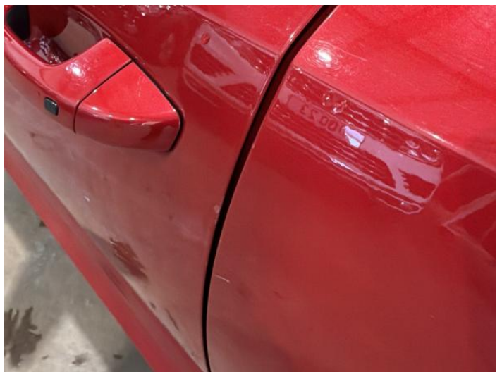
14: Door nsf Chipped Edge Chip
