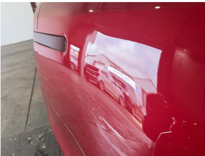
7: Qtr Panel osr Dented Over 30mm
