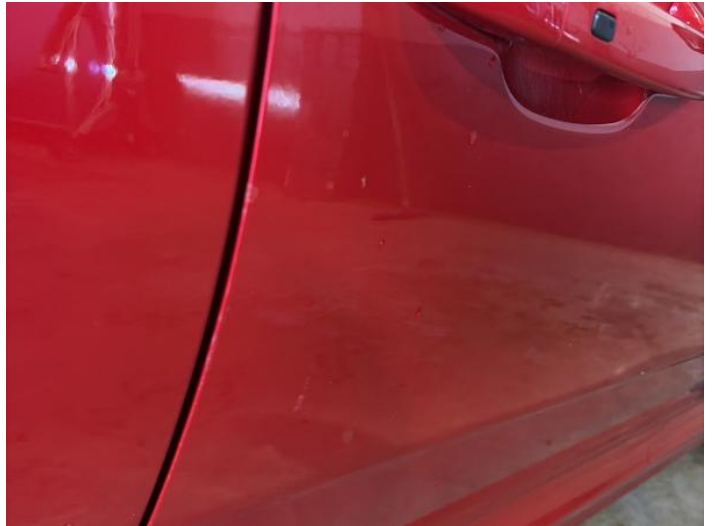
4: Door osf Chipped Edge Chip
