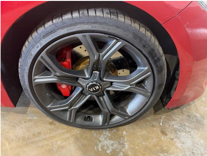
1: Wheel of Scratched Over 50mm
