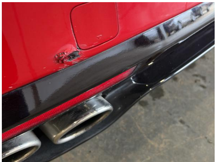
8: Bumper Rear Dented With Paint Damage
