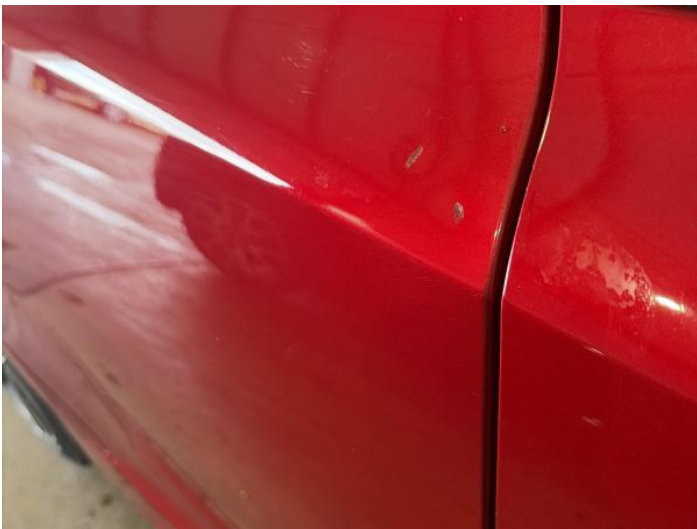
5: Door osr Dented With Paint Damage
