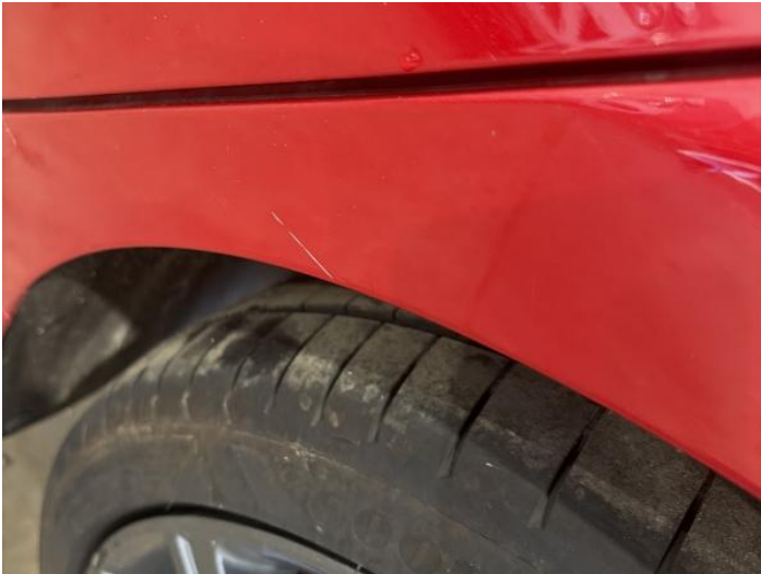
9: Qtr Panel nsr Scratched UpTo 25mm Thru Paint
