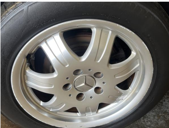
7: Wheel nsf Scratched Over 50mm
