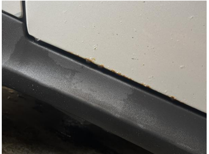
10: Door nsf Rusted Over 5mm
