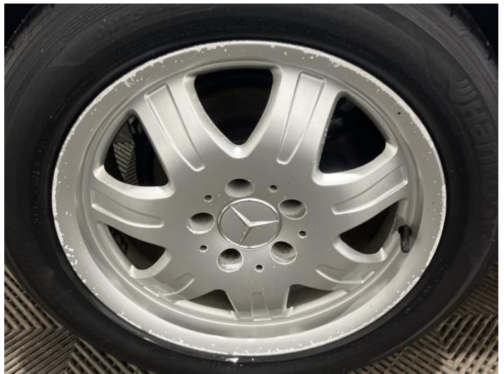
18: Wheel osr Scratched Over 50mm
