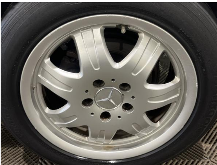
13: Wheel nsr Scratched Over 50mm
