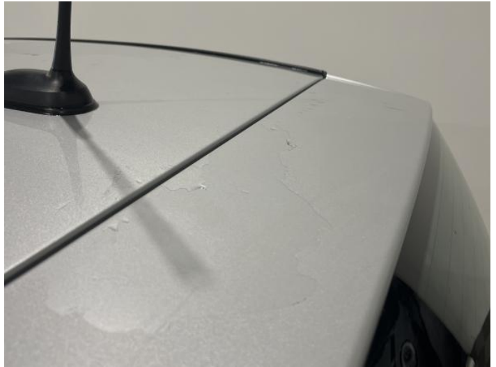
16: Tailgate Poor Previous Repair Paint Flake
