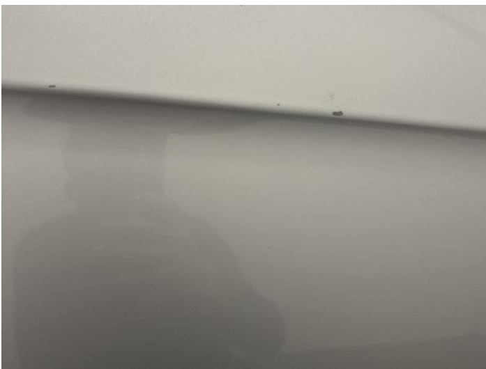
19: Door osr Chipped Multiple Chips
