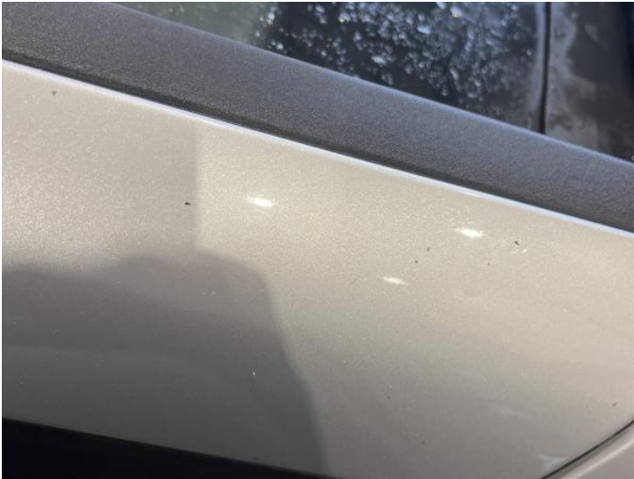
3: A Post os Chipped Multiple Chips
