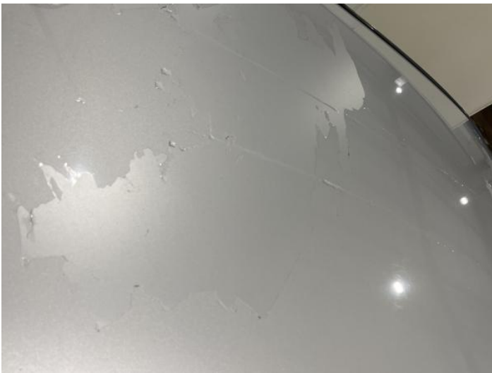
17: Roof Poor Previous Repair Paint Flake
