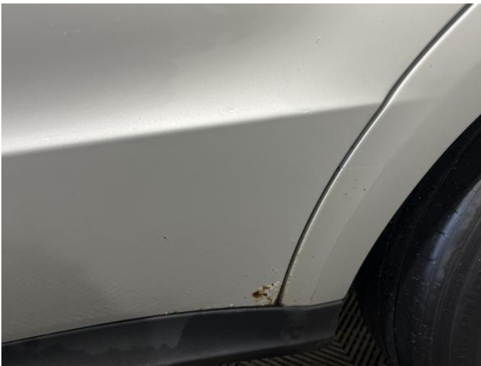
11: Door nsr Rusted Over 5mm
