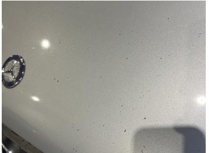
4: Bonnet Chipped Multiple Chips
