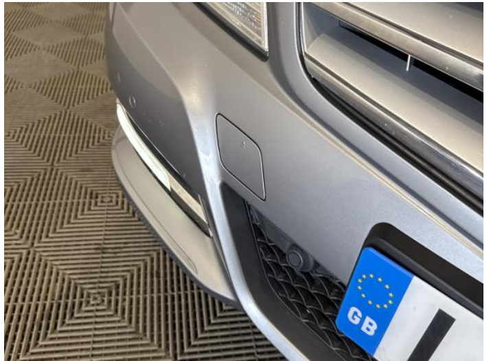
2: Bumper Front Scratched 25 to 100mm Thru Paint
