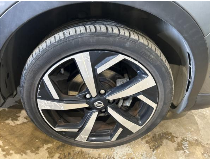
1: Wheel osf Scratched Over 50mm
