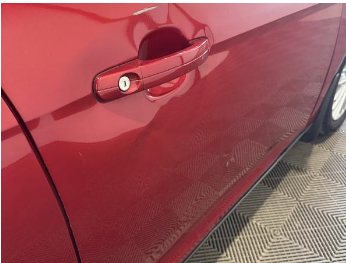
13: Door osf Dented With Paint Damage
