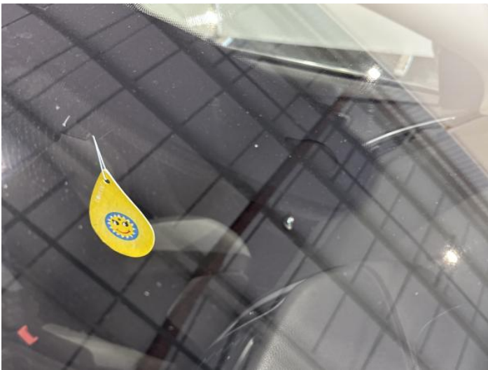
17: Screen Front Chipped Over 10mm
