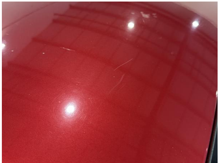
18: Roof Scratched Over 25mm Thru Paint
