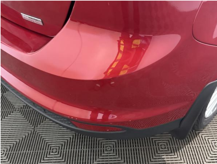
9: Bumper Rear Scratched 25 to 100mm Thru Paint
