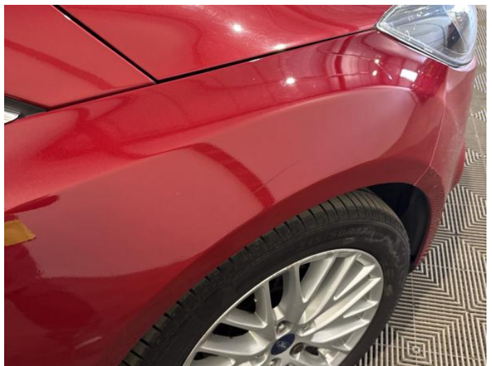
14: Wing osf Poor Previous Repair Poor Paint
