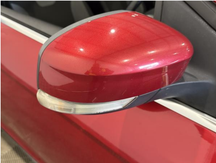
15: Door Mirror Assy osf Scratched (Painted) Over 25mm Thru Paint
