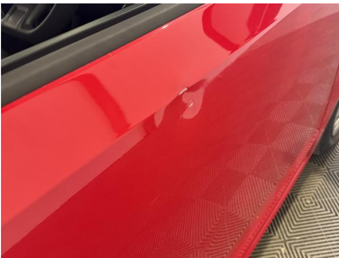
13: Door osf Dented With Paint Damage
