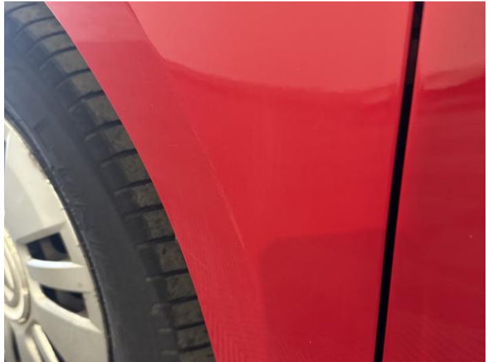
4: Wing nsf Scratched Over 25mm Thru Paint
