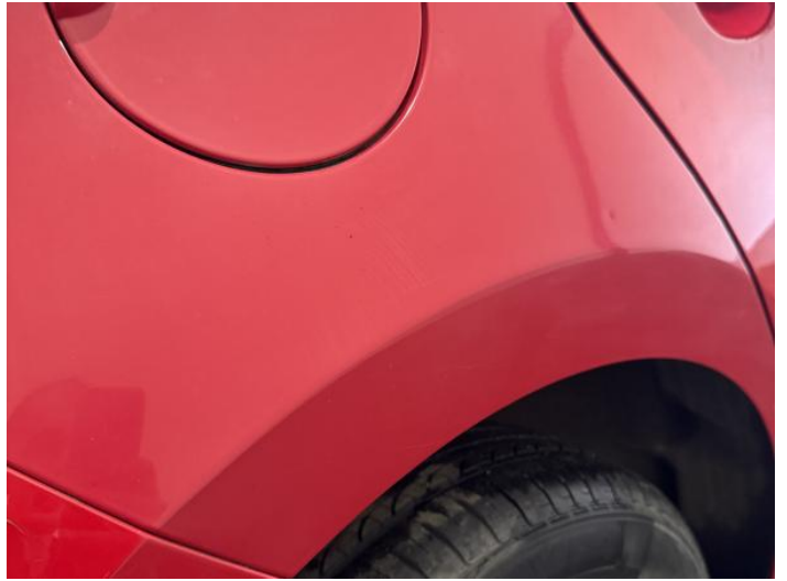
10: Qtr Panel osr Poor Previous Repair Poor Paint
