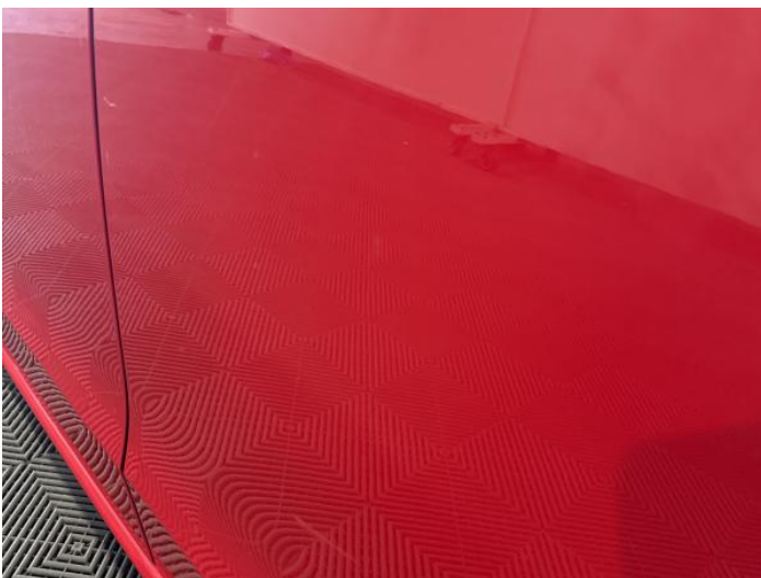
7: Door nsr Scratched Over 25mm Thru Paint
