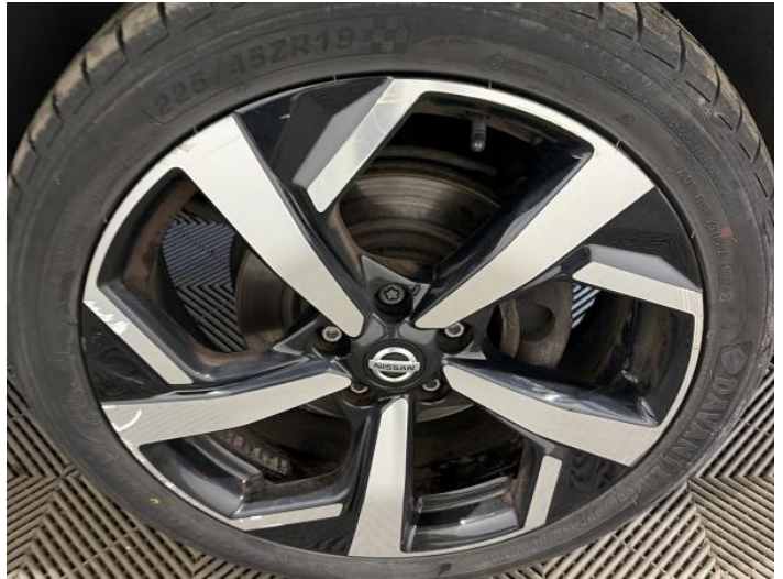
16: Wheel osf Scratched Over 50mm
