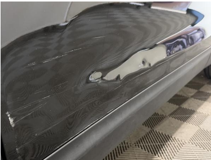
5: Door nsf Dented With Paint Damage
