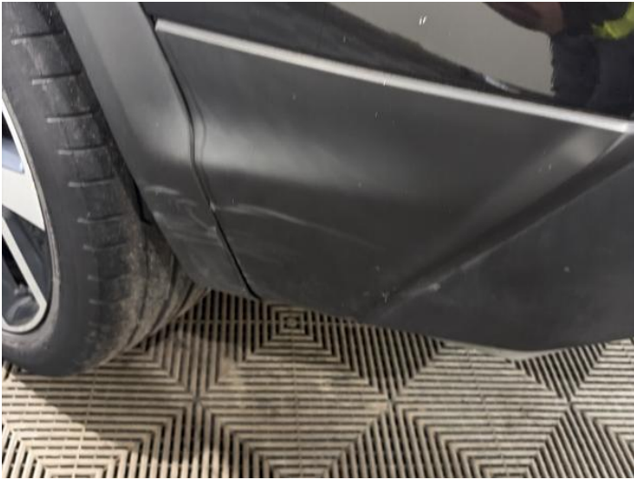
9: Bumper Rear Moulding Scuffed (Unpainted) Over 100mm
