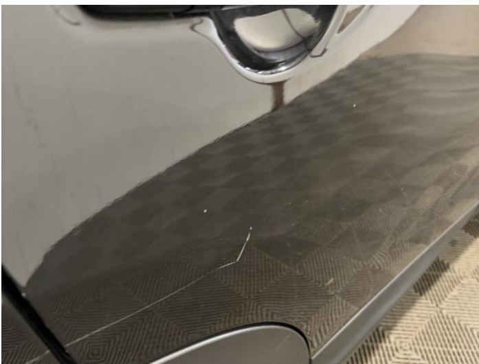
13: Door osr Scratched Over 25mm Thru Paint
