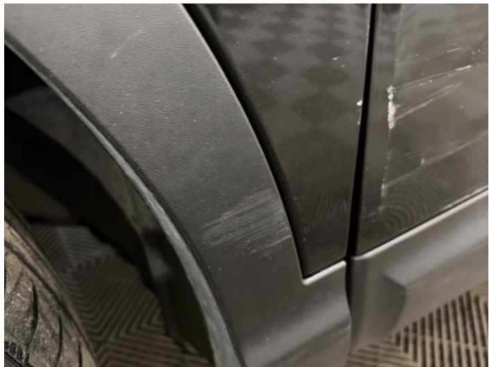
6: Wing Front Arch Extension ns Scuffed (Unpainted) Up To 100mm
