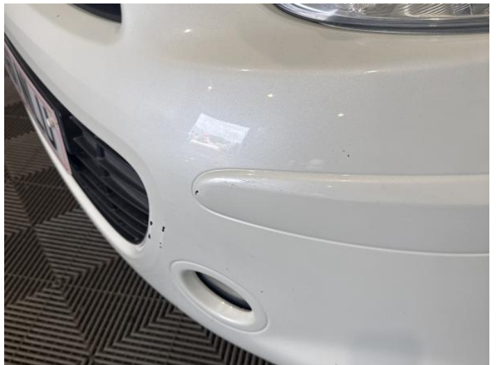
2: Bumper Front Scratched 25 to 100mm Thru Paint
