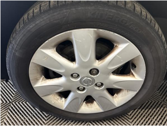
3: Wheel nsf Scratched Over 50mm
