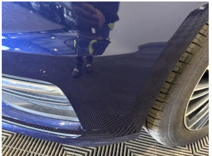
2: Bumper Front Scratched 25 to 100mm Thru Paint
