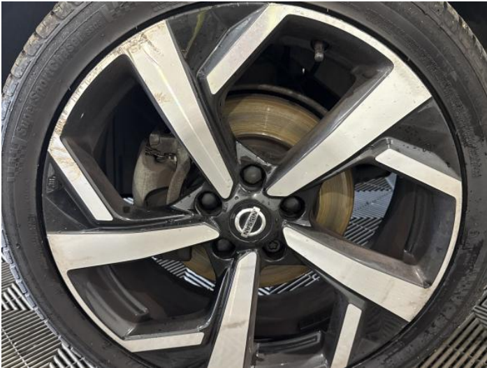
3: Wheel nsf Scratched Over 50mm
