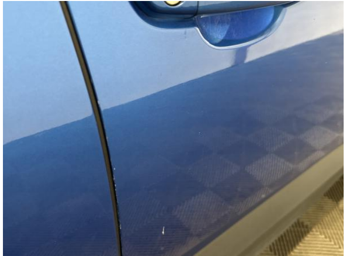
16: Door osf Chipped Edge Chip
