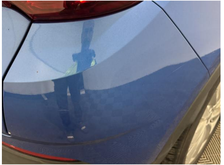
10: Bumper Rear Scratched 25 to 100mm Thru Paint
