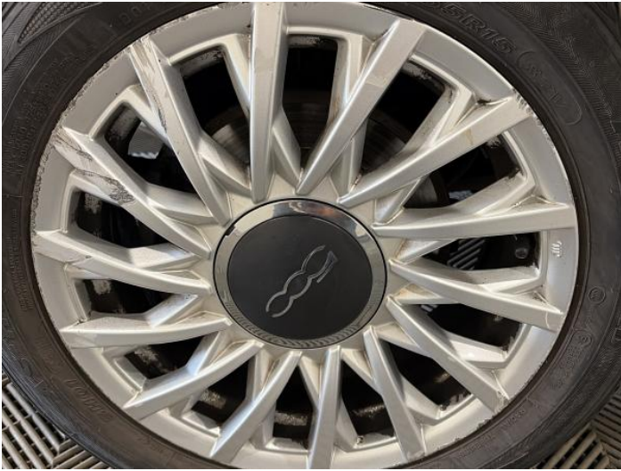
3: Wheel nsf Scratched Over 50mm
