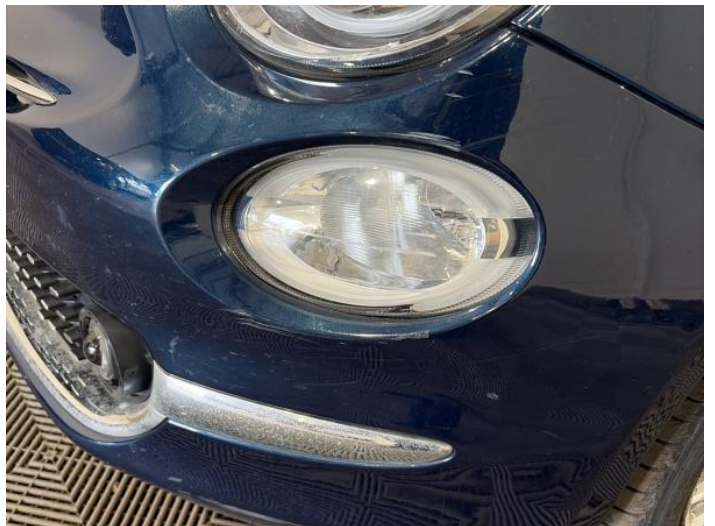
2: Bumper Front Scratched 25 to 100mm Thru Paint
