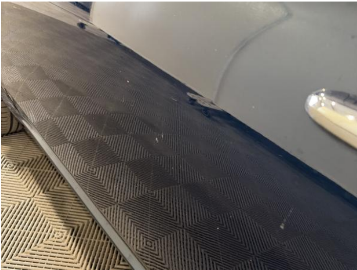
5: Door nsf Scratched Over 25mm Thru Paint
