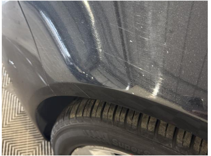
4: Wing nsf Scratched Over 25mm Thru Paint
