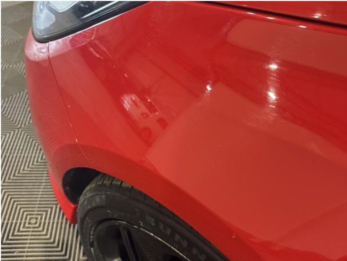
3: Wing nsf Poor Previous Repair Poor Paint
