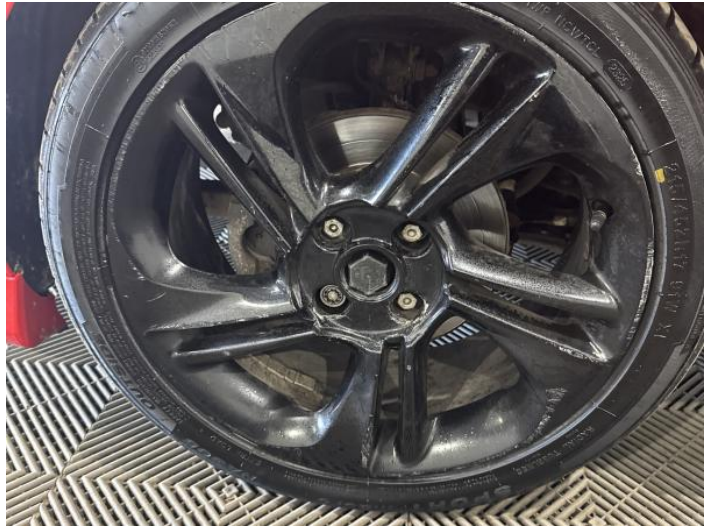
4: Wheel nsf Scratched Over 50mm
