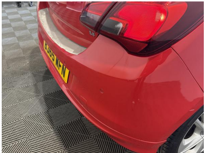
12: Bumper Rear Scratched 25 to 100mm Thru Paint
