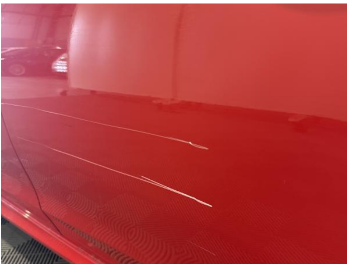
7: Door nsr Scratched Over 25mm Thru Paint
