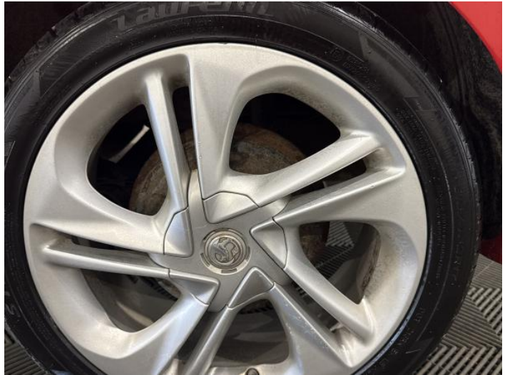
10: Wheel nsr Scratched Over 50mm
