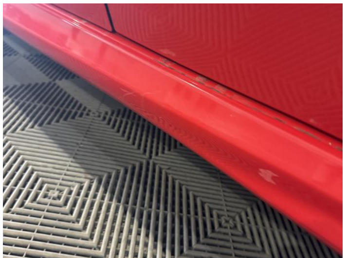
8: Sill Panel Trim ns Scratched (Painted) UpTo 25mm Thru Paint
