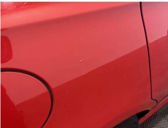
13: Qtr Panel osr Chipped 1 To 5
