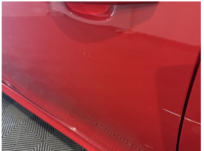
6: Door nsf Scratched Over 25mm Thru Paint
