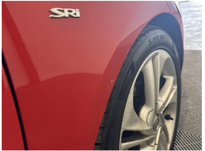
18: Wing osf Poor Previous Repair Paint Flake
