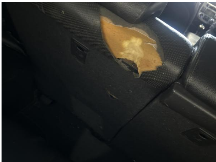
21: Seat Back Cover nsr Holed Over 3mm
