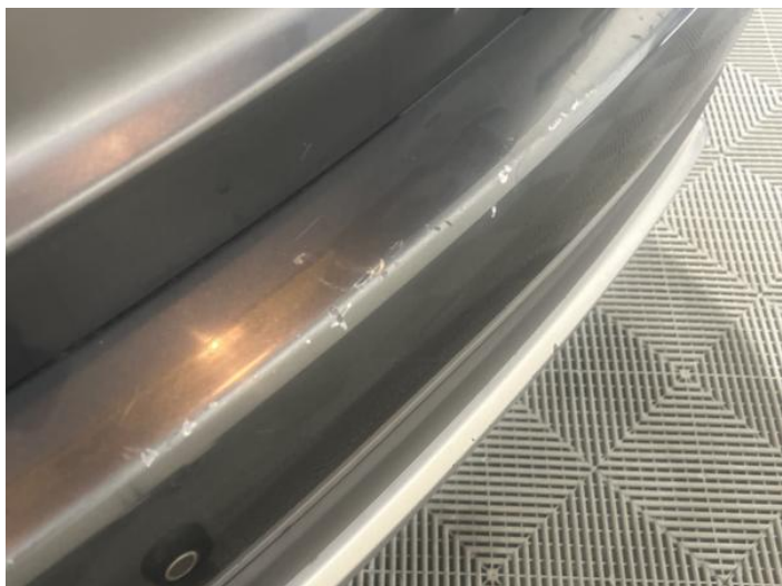
9: Bumper Rear Scratched Over 100mm Thru Paint
