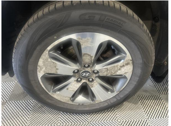
16: Wheel nsf Corroded Light
