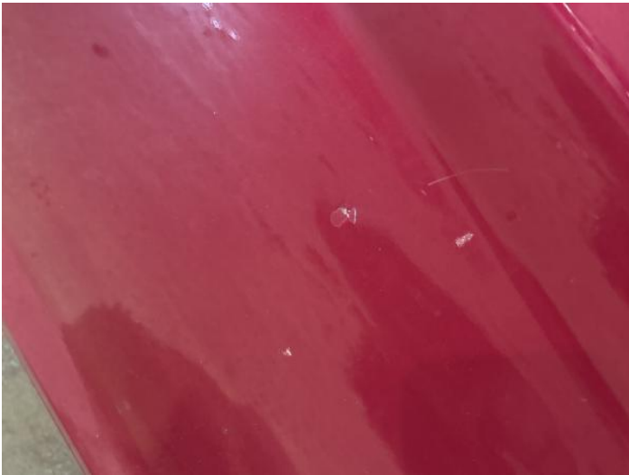
5: Door osf Poor Previous Repair Poor Paint
