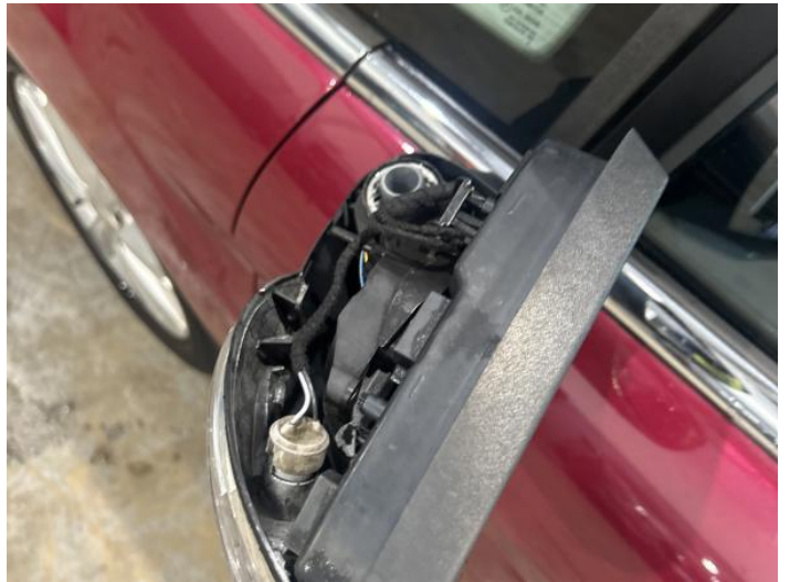
12: Door Mirror Assy nsf Missing Replace
