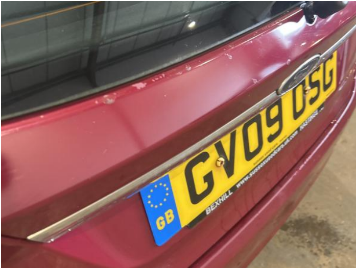
9: Tailgate Poor Previous Repair Paint Flake
