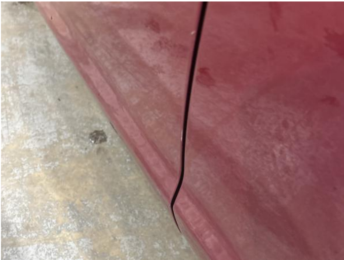
11: Door nsf Chipped Edge Chip
