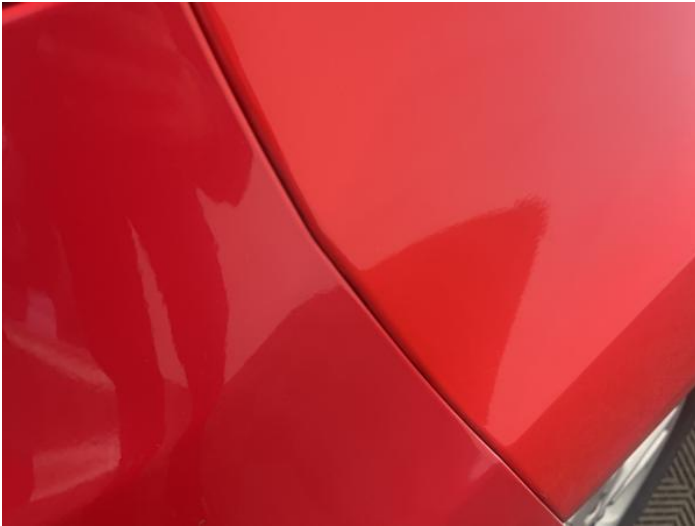
9: Bumper Rear Poor Previous Repair Poor Paint
