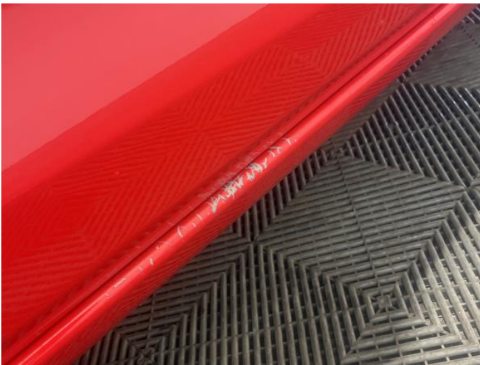
11: Sill os Scratched Over 25mm Thru Paint
