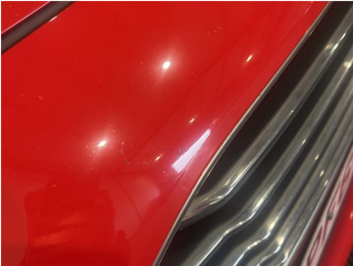
3: Bumper Front Chipped Multiple Chips
