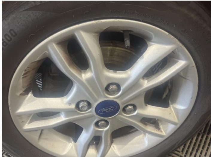
4: Wheel nsf Scratched Up To 50mm
