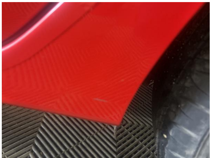
8: Sill ns Scratched Over 25mm Thru Paint
