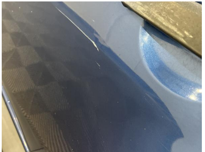
12: Door nsr Scratched Over 25mm Thru Paint
