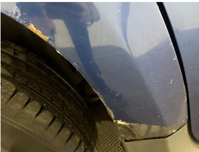
19: Qtr Panel osr Rusted Holed
