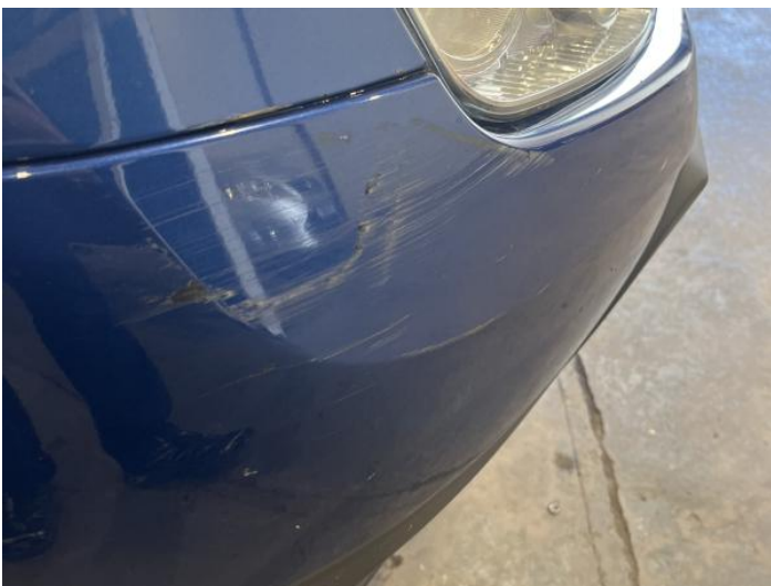
7: Bumper Front Scratched Over 100mm Thru Paint
