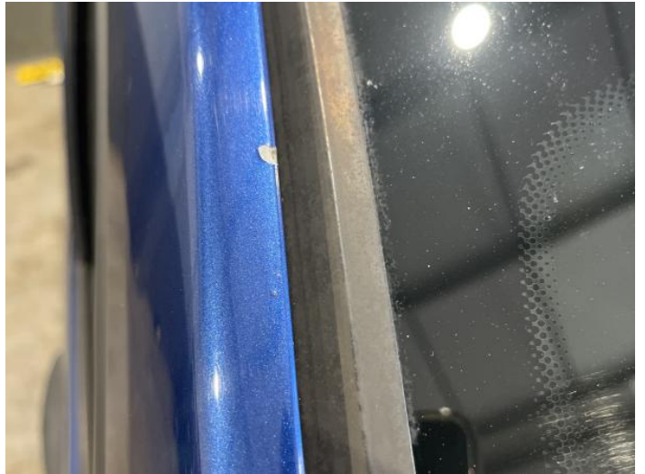
4: A Post os Chipped 1 To 5
