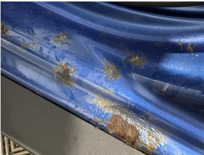
11: Sill ns Rusted Over 5mm
