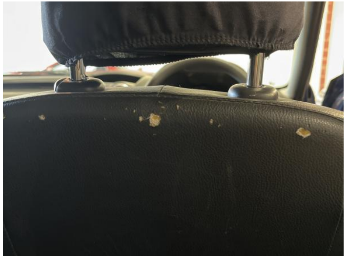
2: Seat Back Cover osf Scuffed UpTo 25mm
