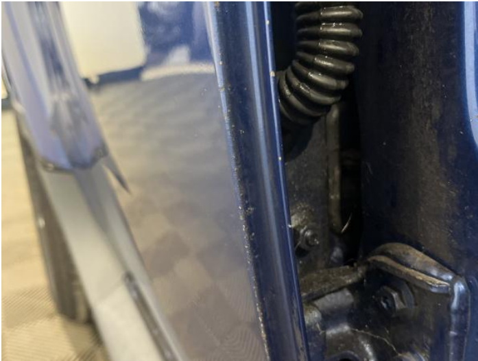
21: Door osr Rusted Over 5mm
