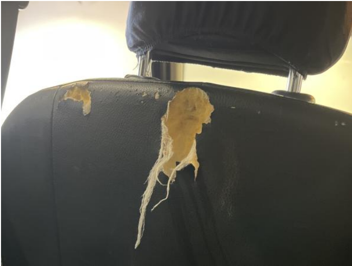
3: Seat Back Cover nsf Torn Over 3mm
