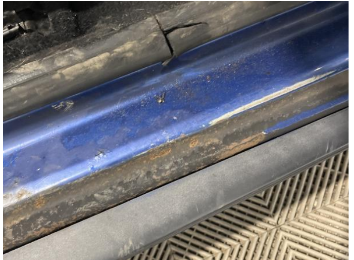
22: Sill os Rusted Over 5mm
