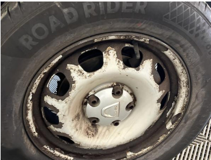
23: Wheel osf Corroded Light
