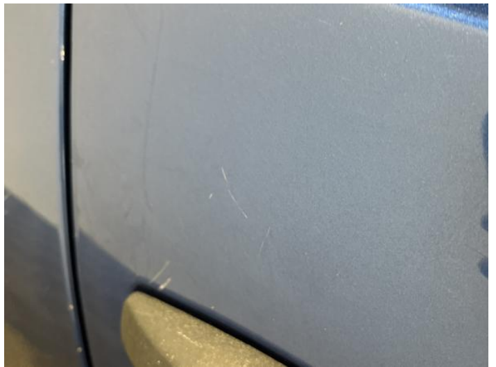
24: Door osf Scratched Over 25mm Thru Paint
