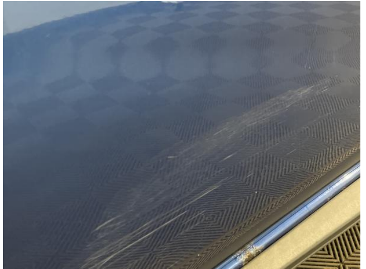
10: Door nsf Scratched Over 25mm Thru Paint
