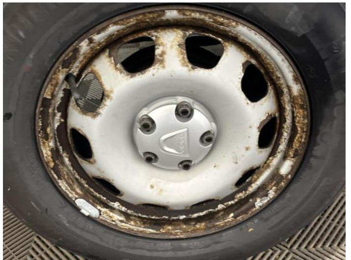
18: Wheel osr Corroded Light
