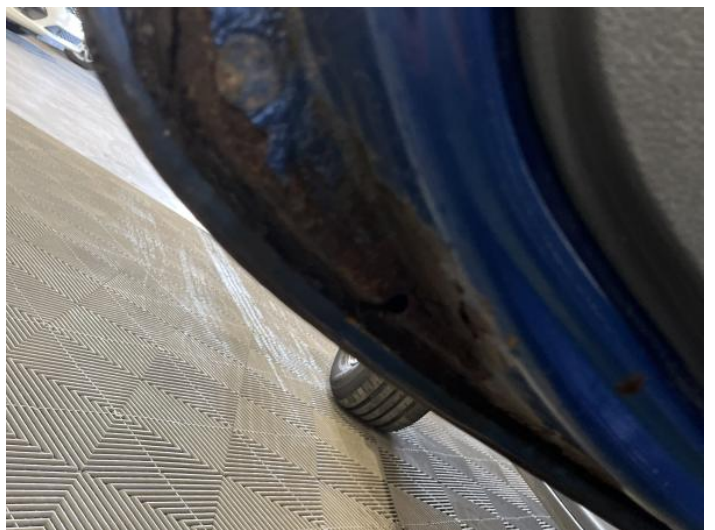
26: Door nsr Rusted Over 5mm
