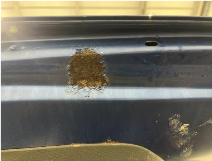
27: Tailgate Rusted Over 5mm
