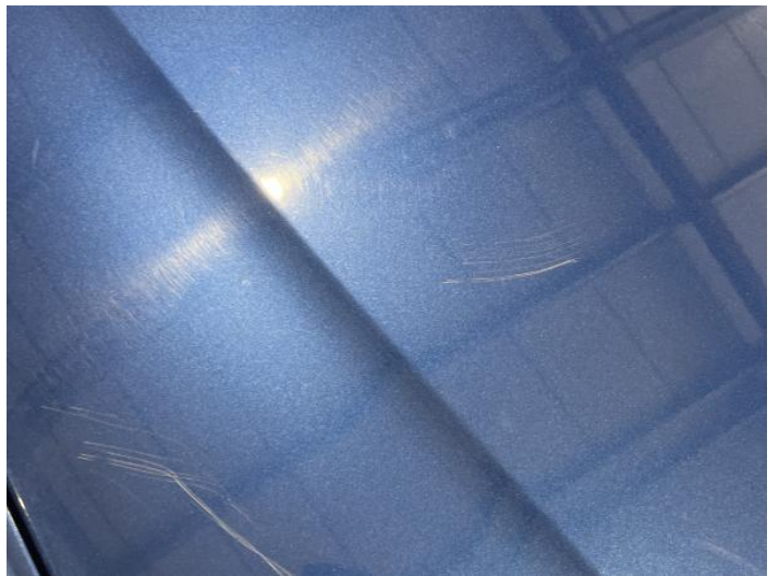
6: Bonnet Scratched Over 25mm Thru Paint
