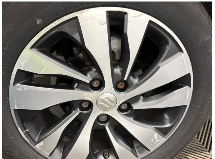
18: Wheel osr Scratched Over 50mm
