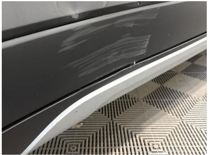
8: Door Moulding nsf Scuffed (Unpainted) Over 100mm
