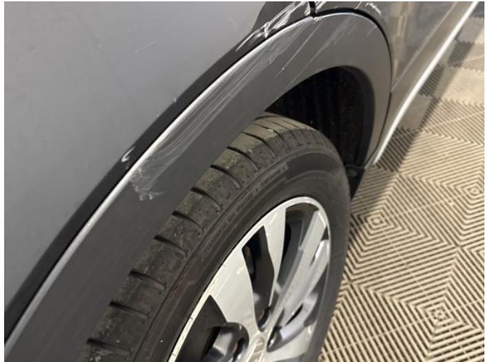
16: Qtr Panel Arch Extension os Scuffed (Unpainted) Over 100mm
