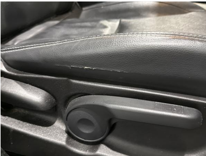
1: Seat Base Cover osf Scuffed Over 25mm
