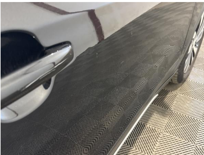
19: Door osf Dented Over 30mm
