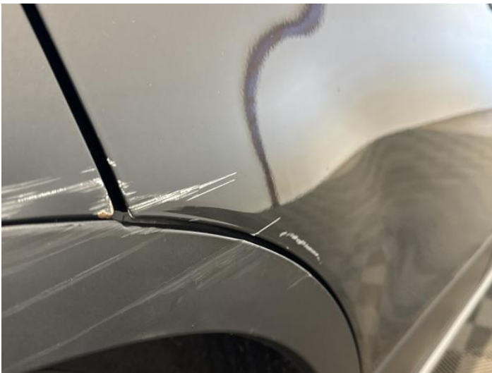
17: Door osr Dented With Paint Damage
