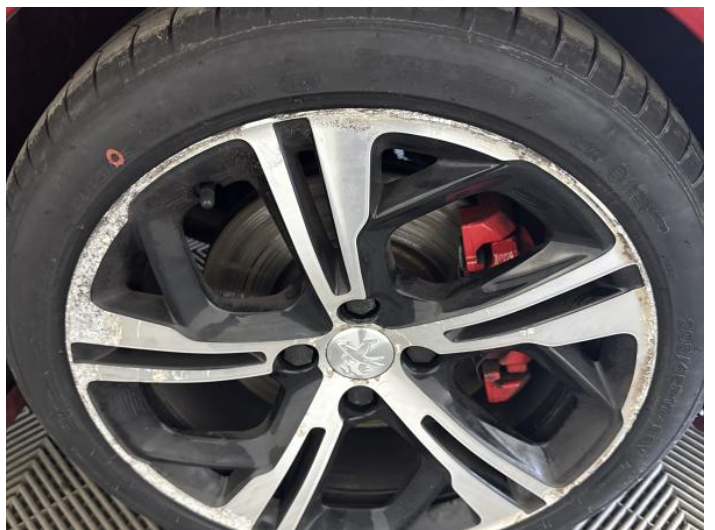
20: Wheel osf Scratched Over 50mm
