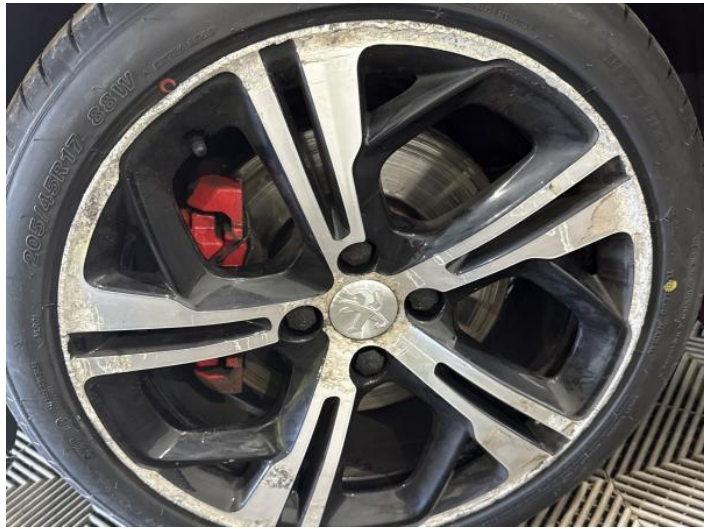
6: Wheel nsf Scratched Over 50mm
