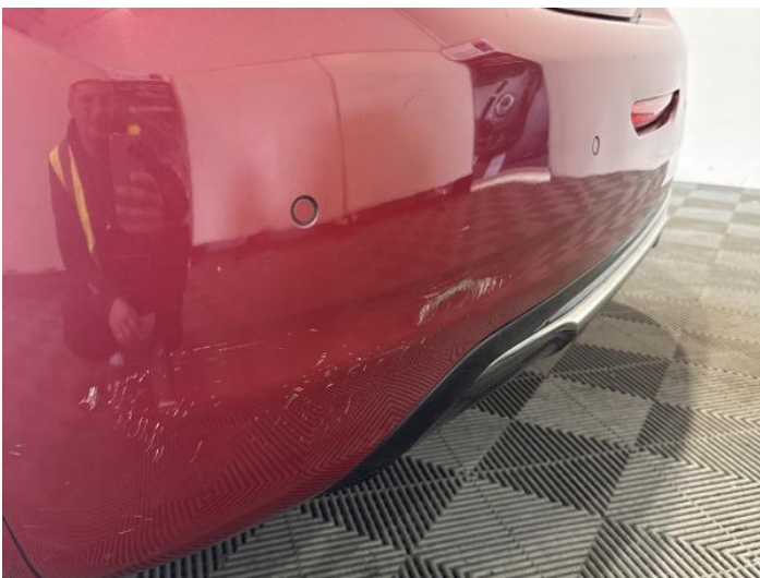
13: Bumper Rear Scratched Over 100mm Thru Paint
