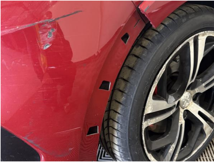
3: Bumper Front Moulding Missing Replace
