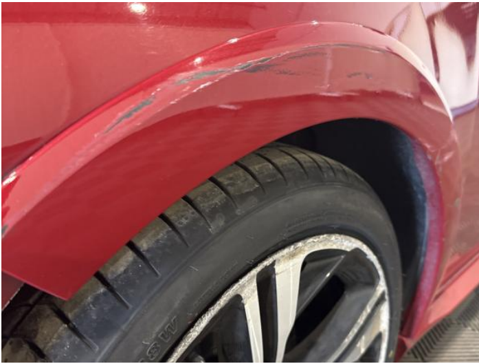
5: Wing Front Arch Extension ns Scratched (Painted) Over 25mm Thru Paint
