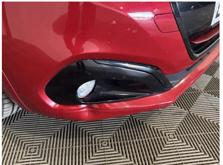
2: Bumper Front Dented With Paint Damage
