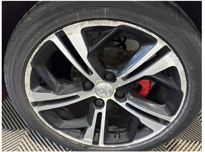
12: Wheel nsr Scratched Over 50mm
