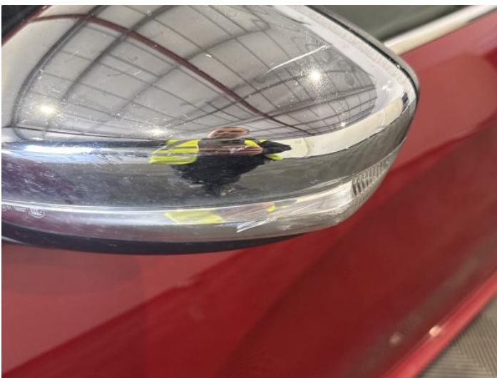
7: Flasher Side Repeater ns Broken Replace
