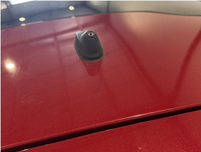
15: Aerial Missing Replace
