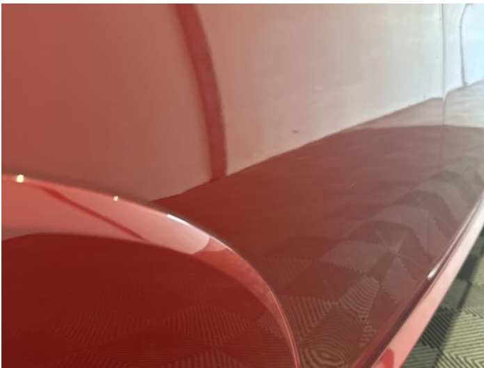
17: Qtr Panel osr Dented Between 10mm + 30mm
