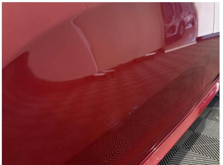
8: Door nsf Dented With Paint Damage
