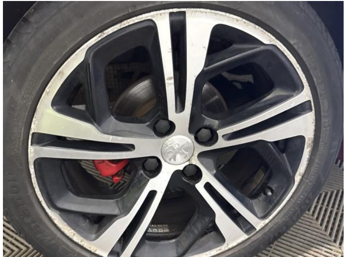
16: Wheel osr Scratched Over 50mm
