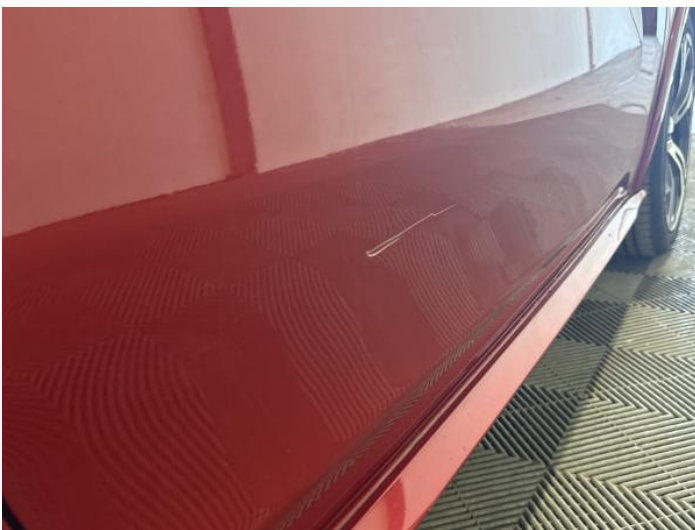
19: Door osf Dented With Paint Damage
