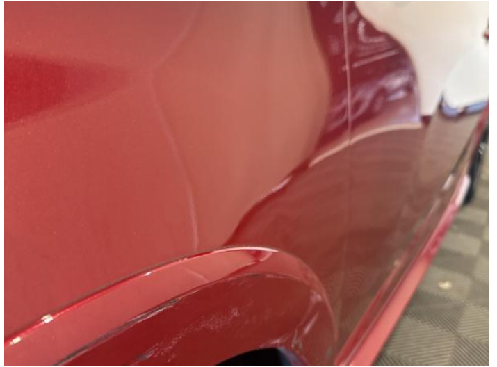
4: Wing nsf Dented Over 30mm
