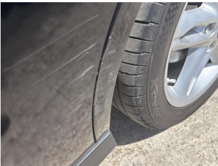
7: Qtr Panel nsr Dented With Paint Damage
