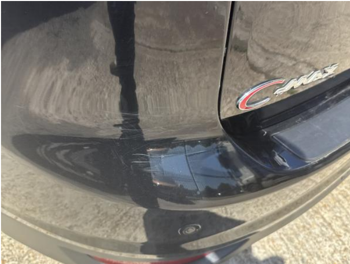
9: Bumper Rear Scratched 25 to 100mm Thru Paint
