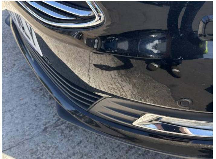
2: Bumper Front Scratched 25 to 100mm Thru Paint
