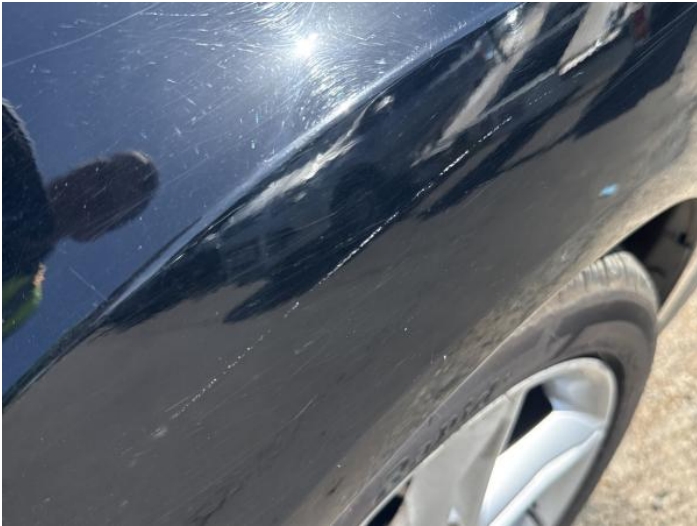
3: Wing nsf Scratched Over 25mm Thru Paint
