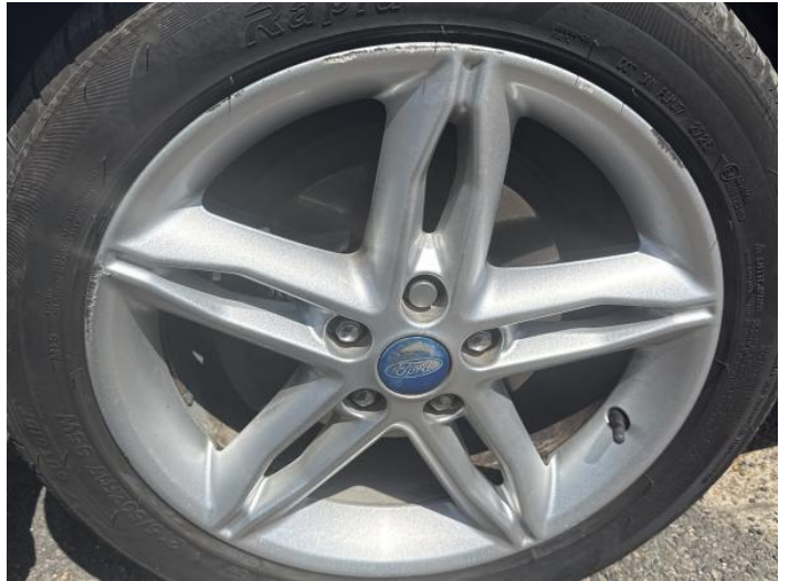
4: Wheel nsf Scratched Over 50mm
