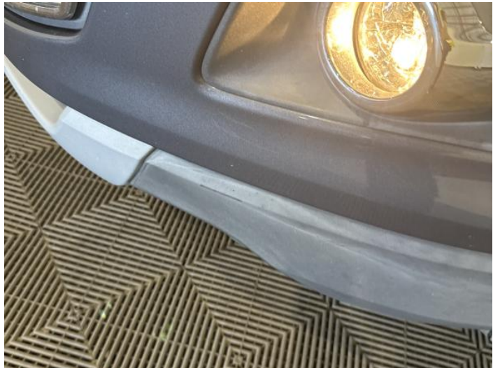
2: Bumper Front Scratched 25 to 100mm Thru Paint
