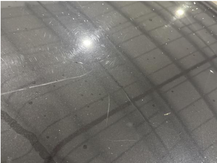
1: Bonnet Scratched Over 25mm Thru Paint
