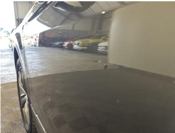
5: Door nsf Dented Over 30mm
