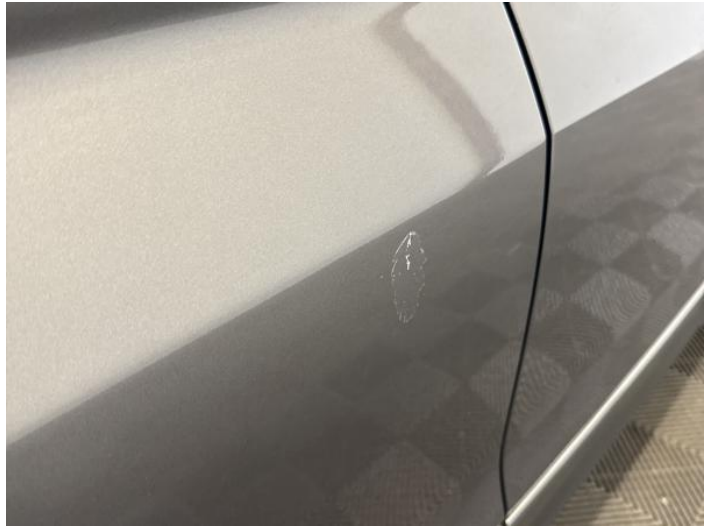
10: Door osr Poor Previous Repair Paint Flake
