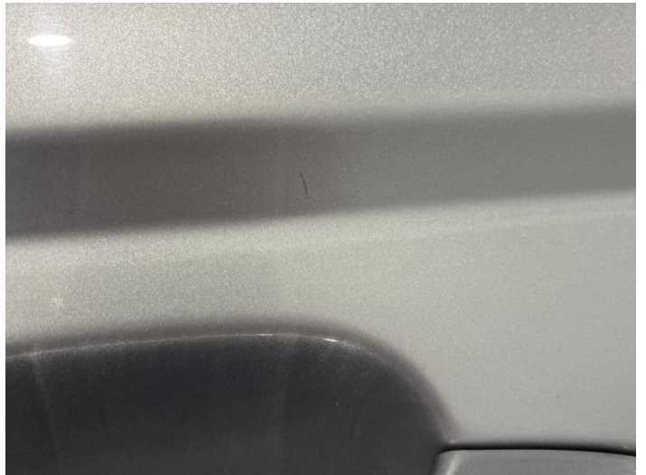
2: Door osf Scratched UpTo 25mm Thru Paint
