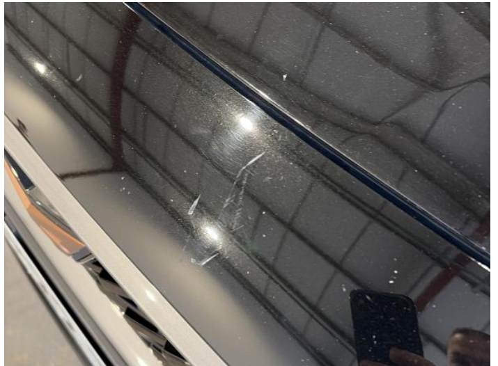
2: Bumper Front Scratched 25 to 100mm Thru Paint
