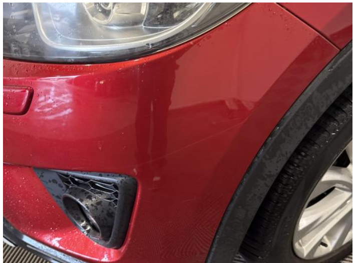
2: Bumper Front Scratched 25 to 100mm Thru Paint
