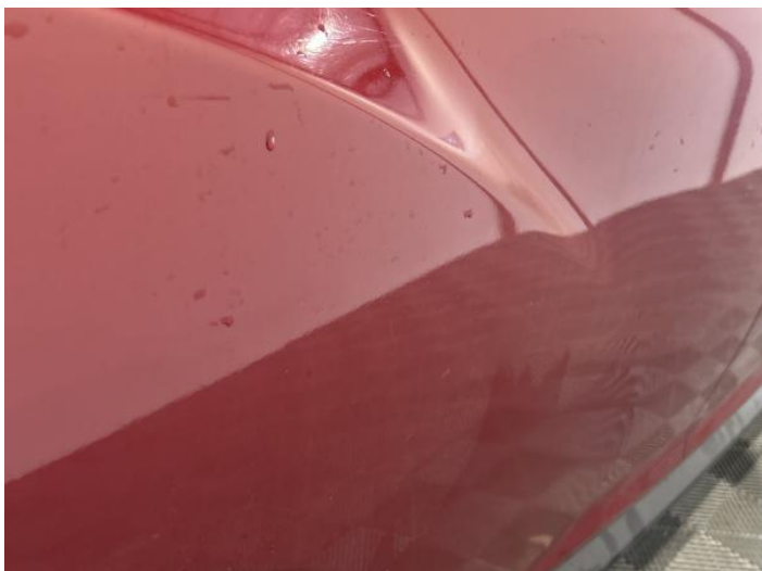
3: Door osr Scratched Over 25mm Not Thru Paint
