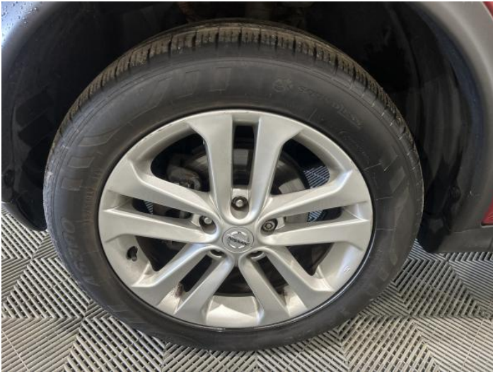
9: Wheel nsf Scratched Over 50mm
