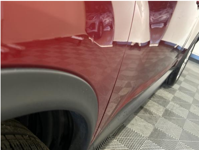
11: Wing nsf Dented 2 Or Less UpTo 10mm
