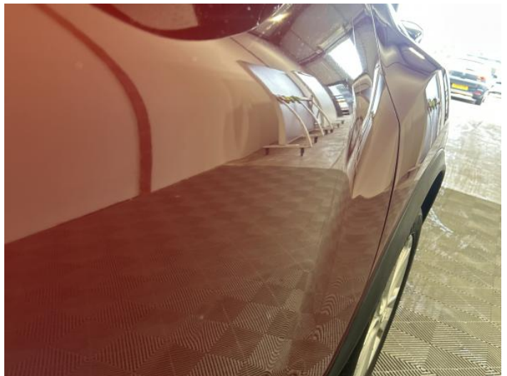
2: Door osf Dented Between 10mm + 30mm
