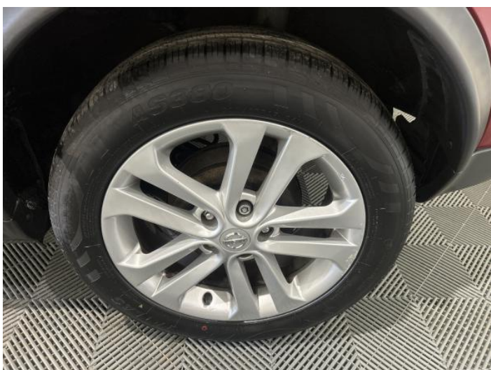
5: Wheel nsr Scratched Over 50mm
