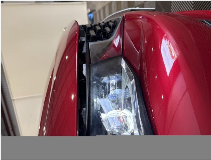
13: Bumper Front Grill Broken Replace
