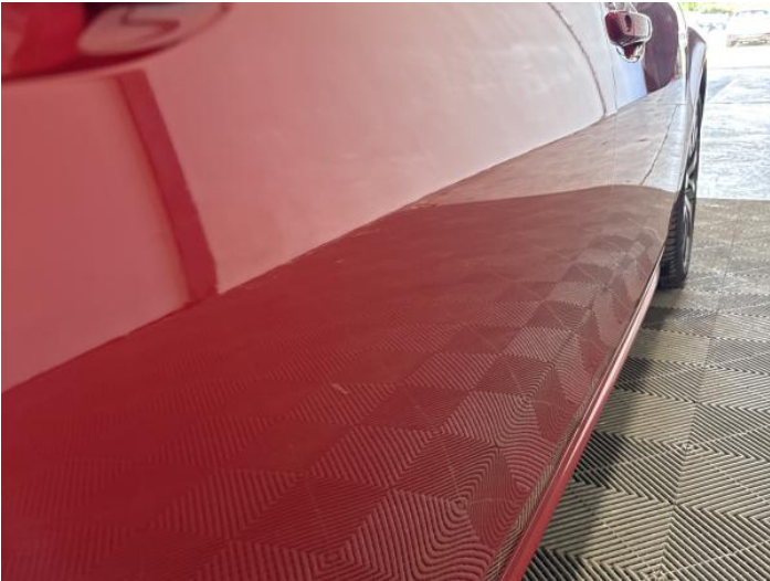
10: Door osr Poor Previous Repair Poor Paint
