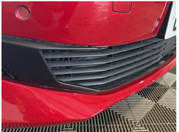
2: Bumper Front Grill Broken Replace
