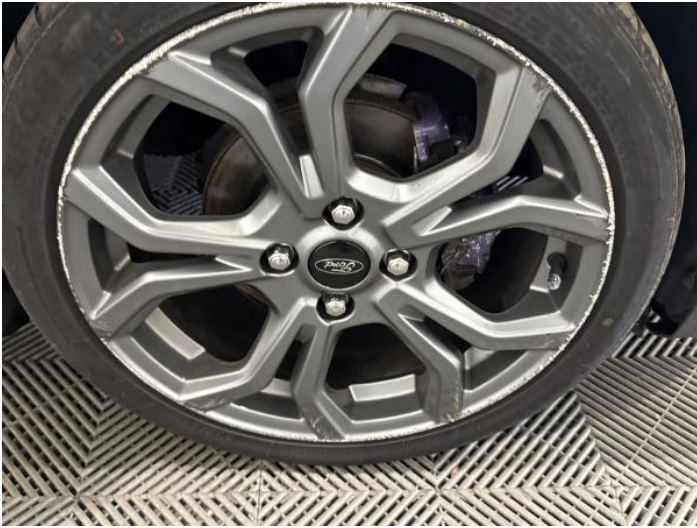
15: Wheel osf Scratched Over 50mm
