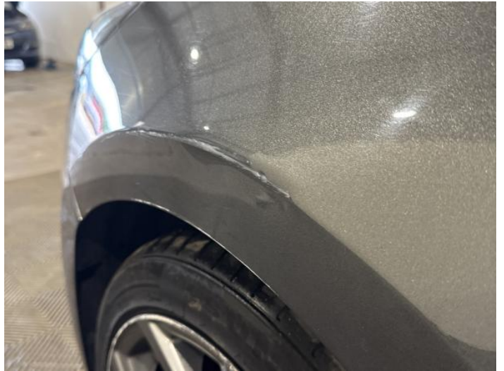
4: Wing nsf Dented With Paint Damage
