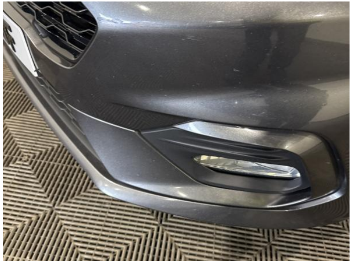
2: Bumper Front Poor Previous Repair Poor Paint
