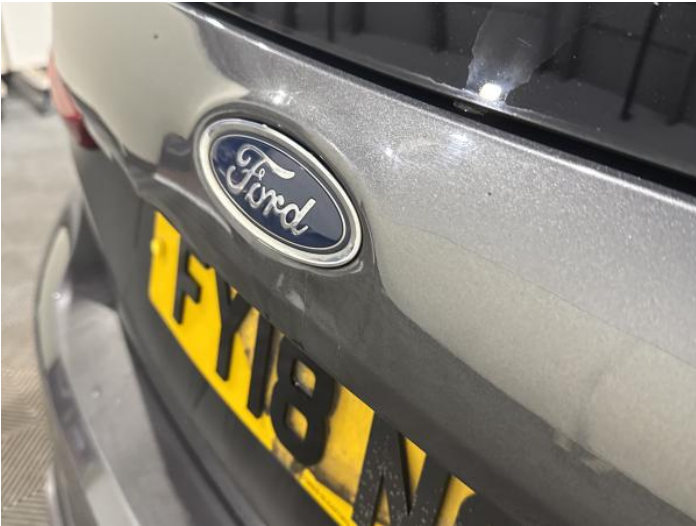
9: Tailgate Dented Over 30mm
