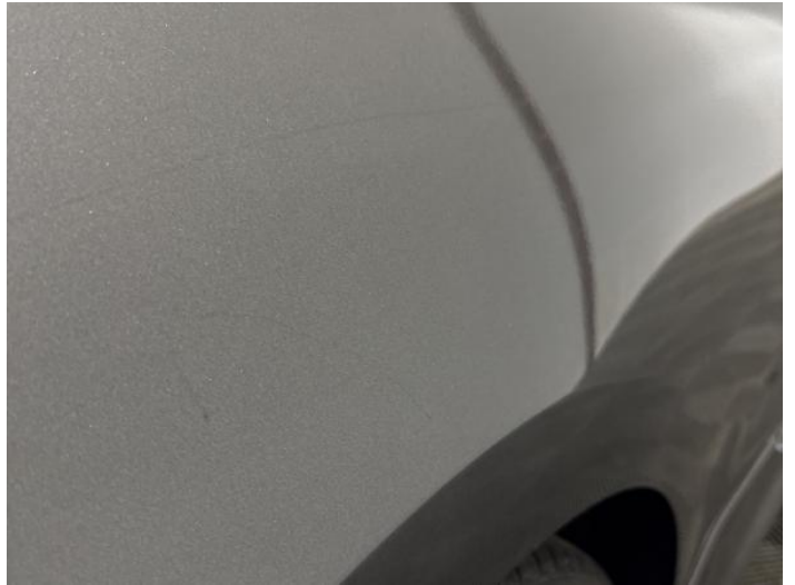
10: Qtr Panel osr Dented Between 10mm + 30mm
