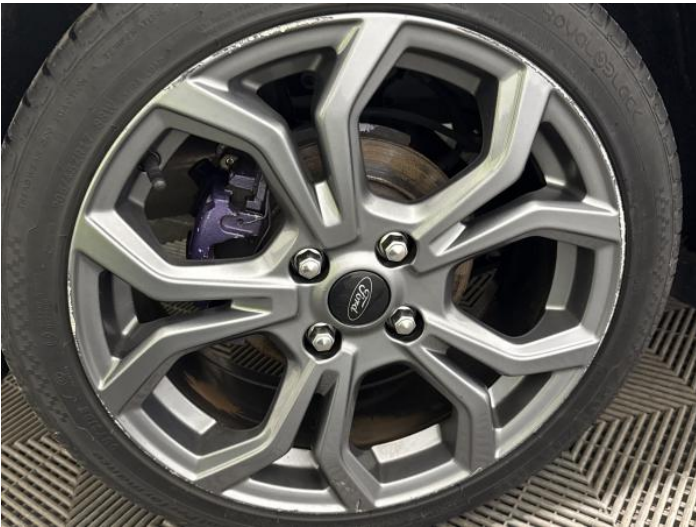
11: Wheel osr Scratched Over 50mm
