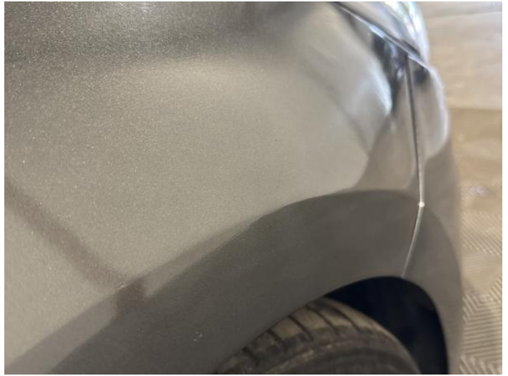
16: Wing nsf Poor Previous Repair Poor Paint
