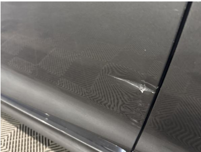
5: Door nsr Dented With Paint Damage
