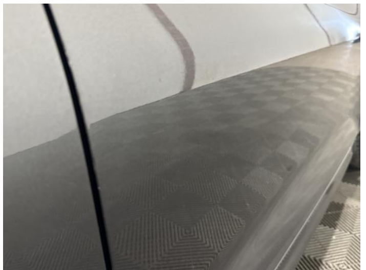
14: Door osf Dented Between 10mm + 30mm
