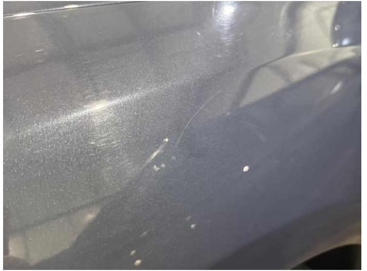
4: Wing nsf Scratched Over 25mm Thru Paint
