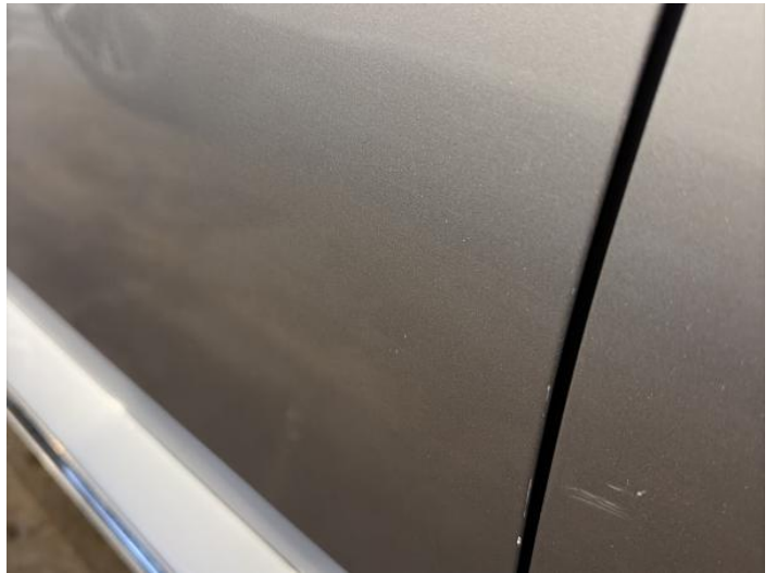
6: Door nsf Chipped Edge Chip
