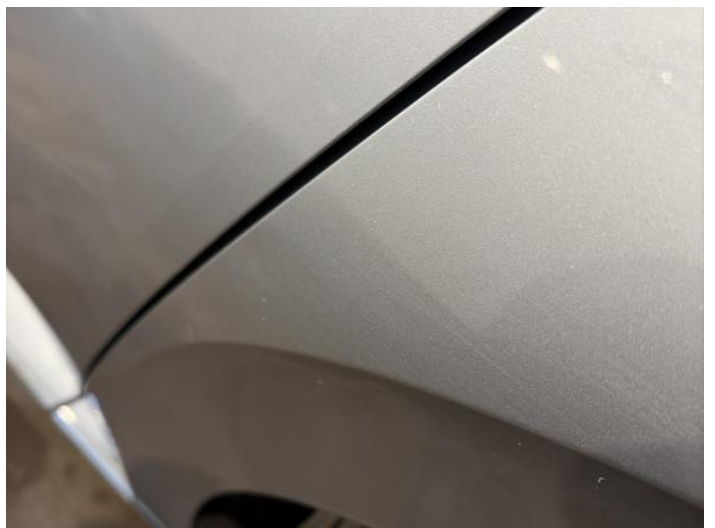
8: Qtr Panel nsr Dented Between 10mm + 30mm
