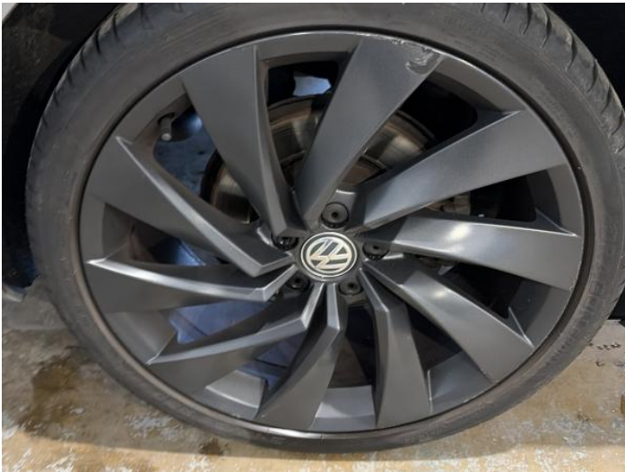
11: Wheel osr Scratched Over 50mm
