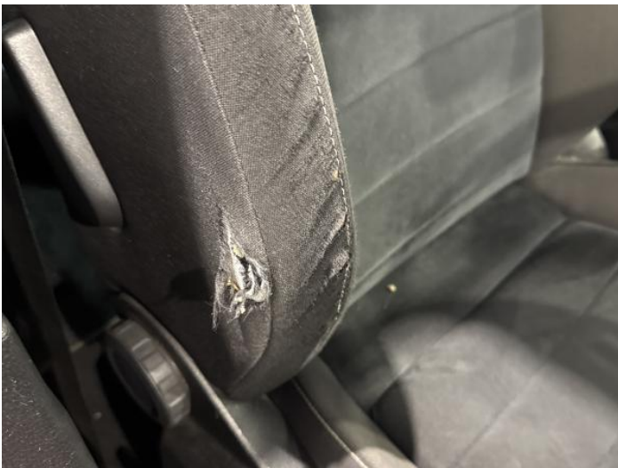
1: Seat Back Cover of Torn Over 3mm
