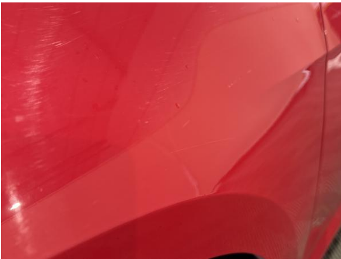
5: Wing nsf Scratched Over 25mm Thru Paint
