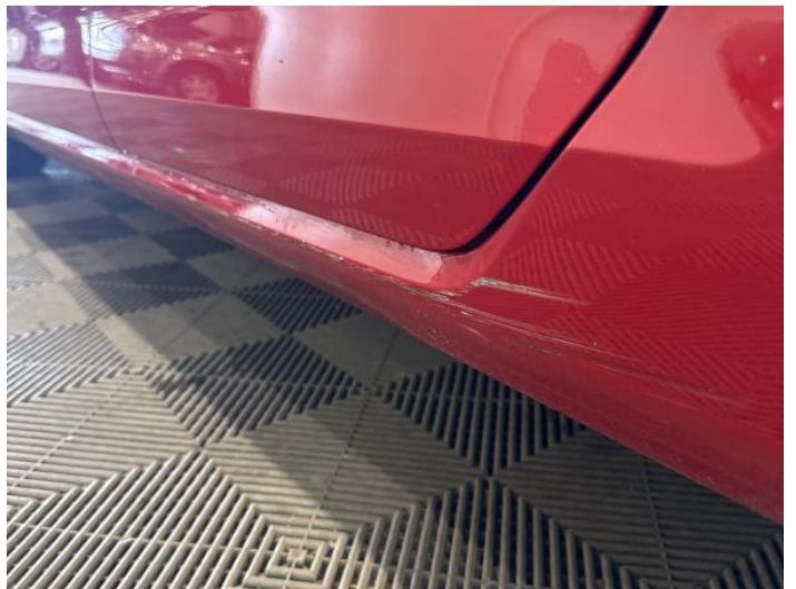
12: Sill ns Scratched Over 25mm Thru Paint
