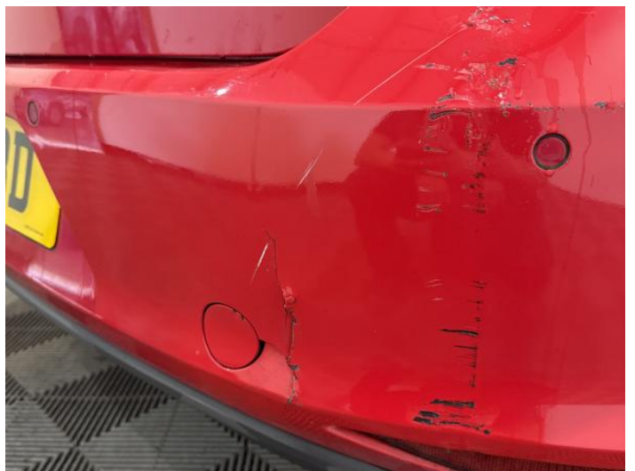
14: Bumper Rear Cracked Over 25mm
