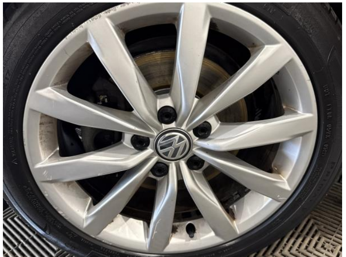
6: Wheel nsf Scratched Over 50mm
