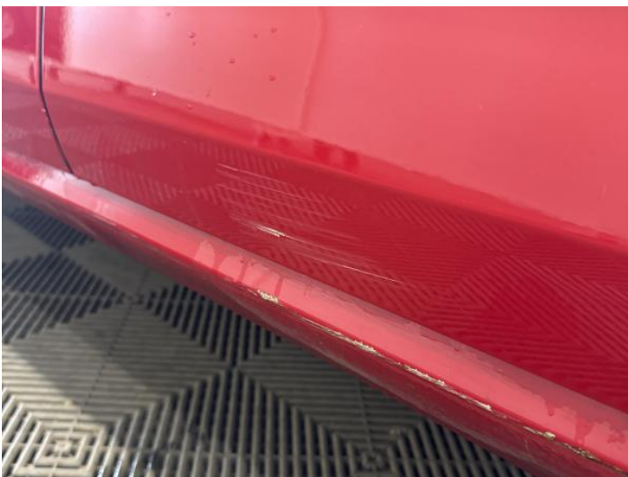
13: Door nsr Scratched Over 25mm Thru Paint
