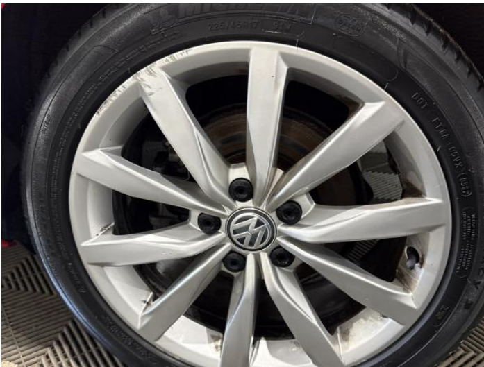
11: Wheel nsr Scratched Over 50mm
