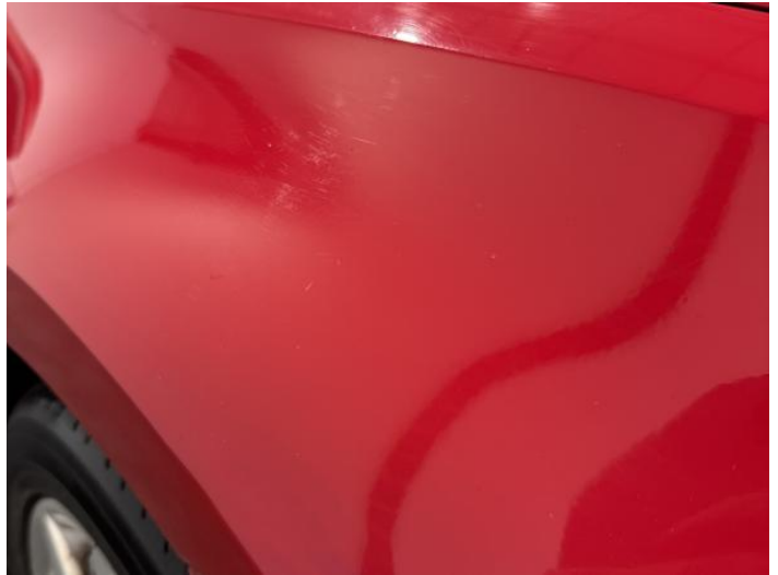
4: Wing osf Poor Previous Repair Poor Paint
