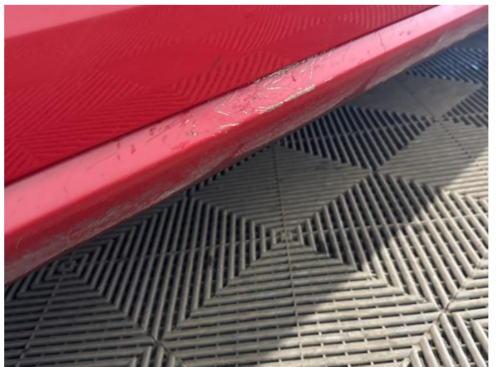
20: Sill os Scratched Over 25mm Thru Paint
