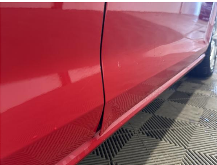
19: Door osf Dented Over 30mm
