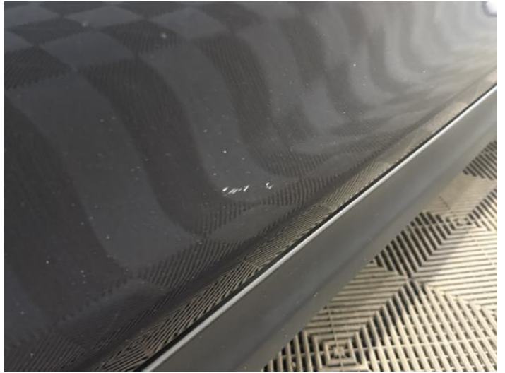
4: Door nsf Scratched Over 25mm Thru Paint
