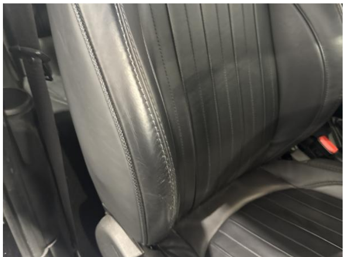
14: Seat Back Cover osf Scuffed Over 25mm
