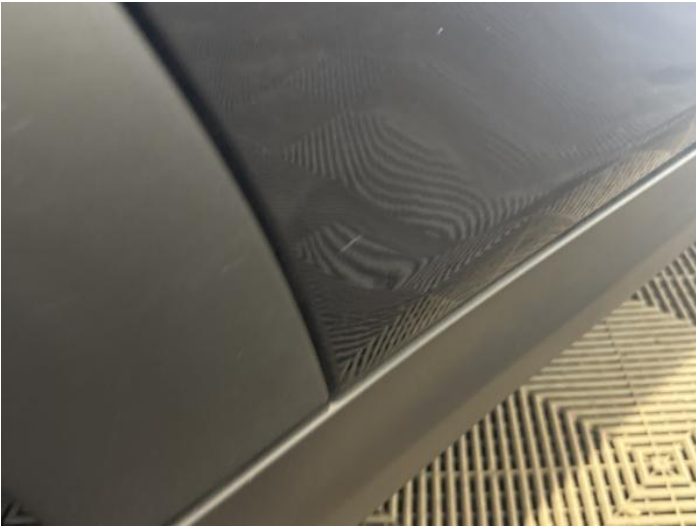
9: Qtr Panel osf Scratched UpTo 25mm Thru Paint
