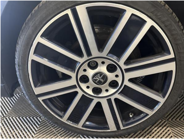
3: Wheel nsf Scratched Over 50mm
