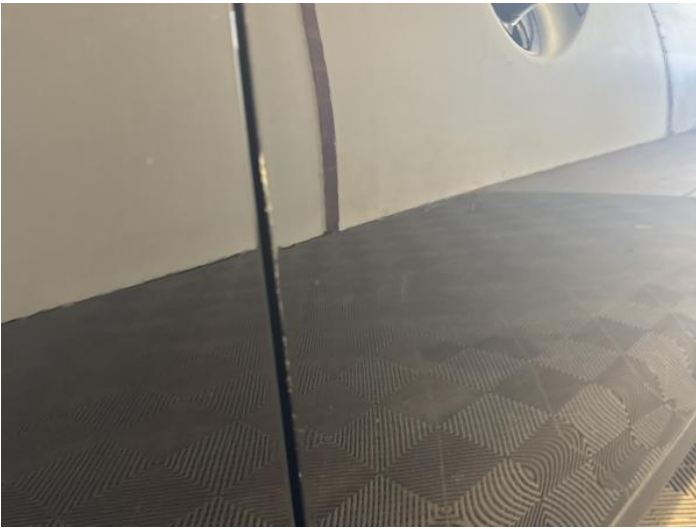
11: Door osf Chipped Edge Chip
