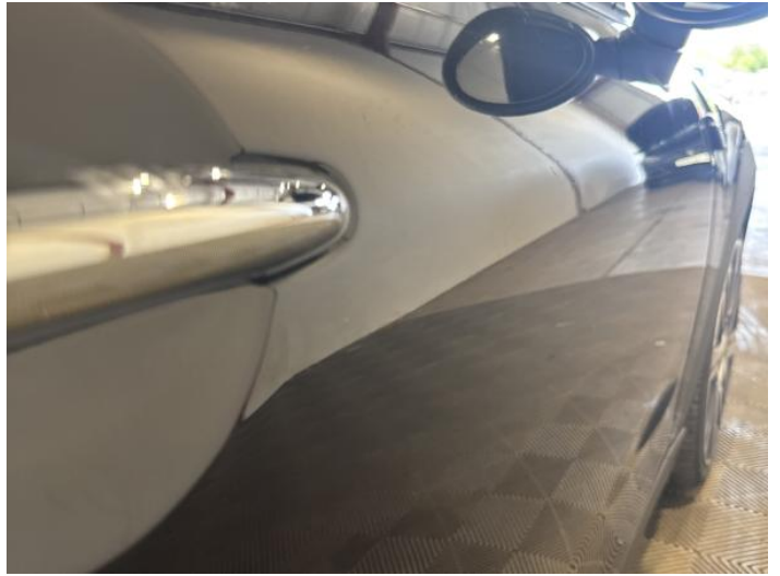
10: Door osf Dented Between 10mm + 30mm
