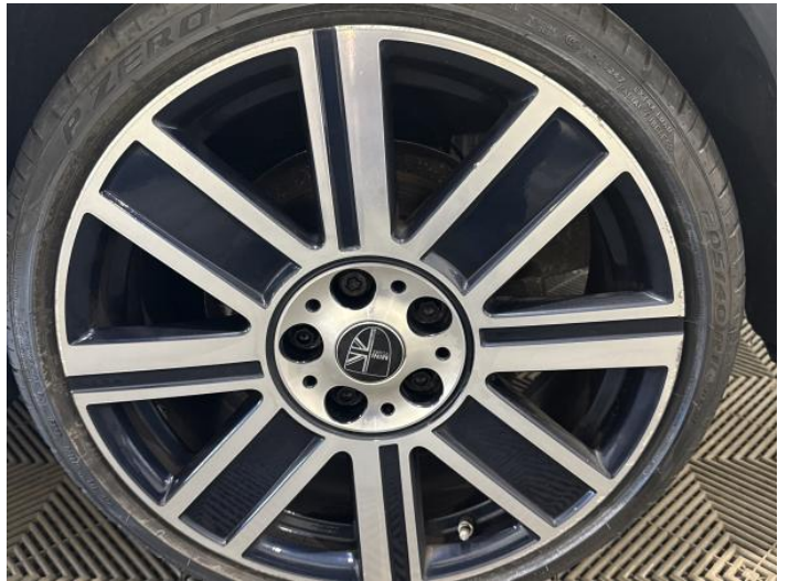
6: Wheel nsr Scratched Over 50mm
