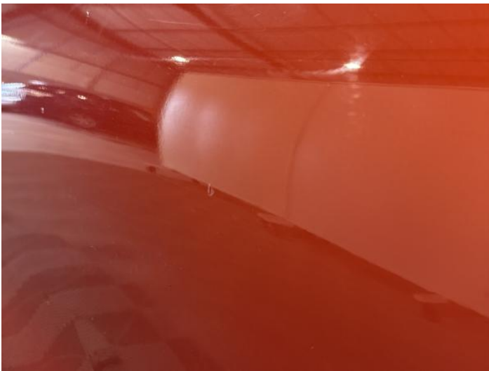
5: Door nsr Scratched Up To 25mm Thru Paint
