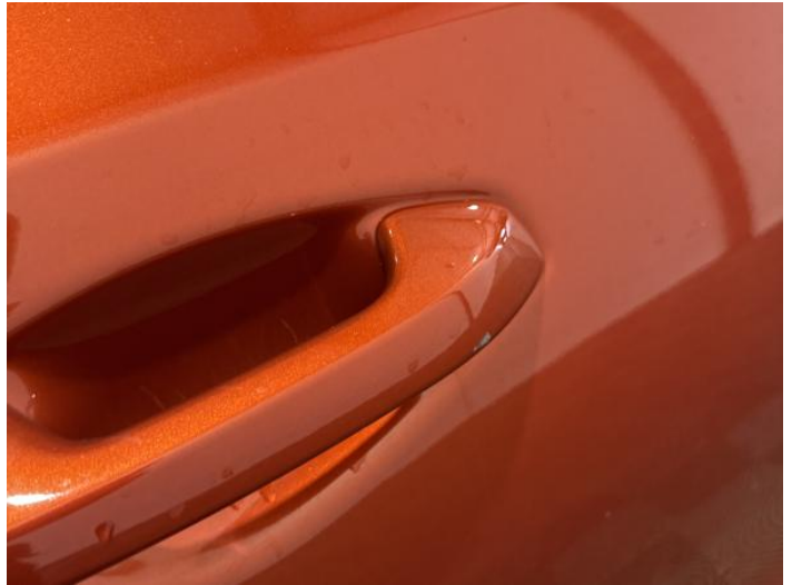
10: Handle Outer osf Scratched (Painted) UpTo 25mm Thru Paint
