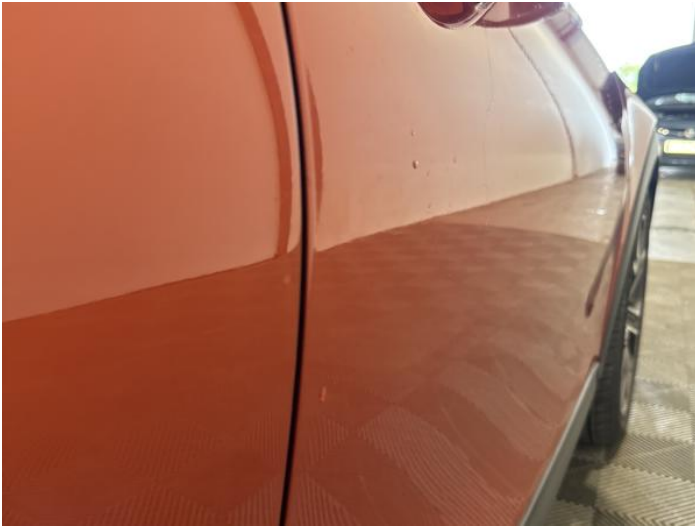
9: Door osf Dented Over 30mm
