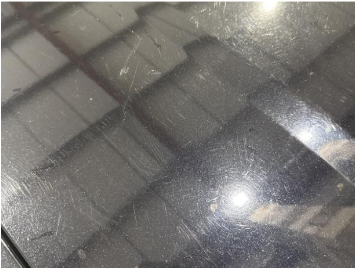
1: Bonnet Scratched Over 25mm Thru Paint
