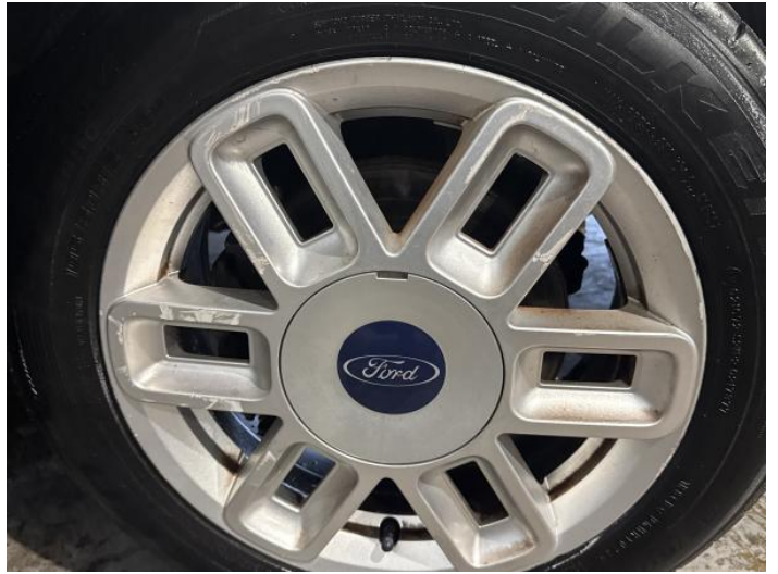
4: Wheel nsf Scratched Over 50mm
