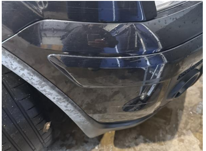
2: Bumper Front Scratched 25 to 100mm Thru Paint
