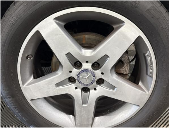
9: Wheel nsr Scratched Over 50mm
