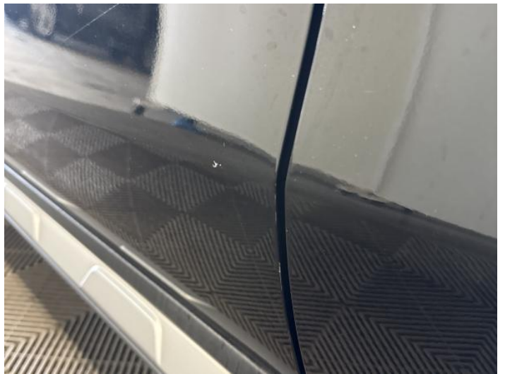
6: Door nsf Chipped 1 To 5
