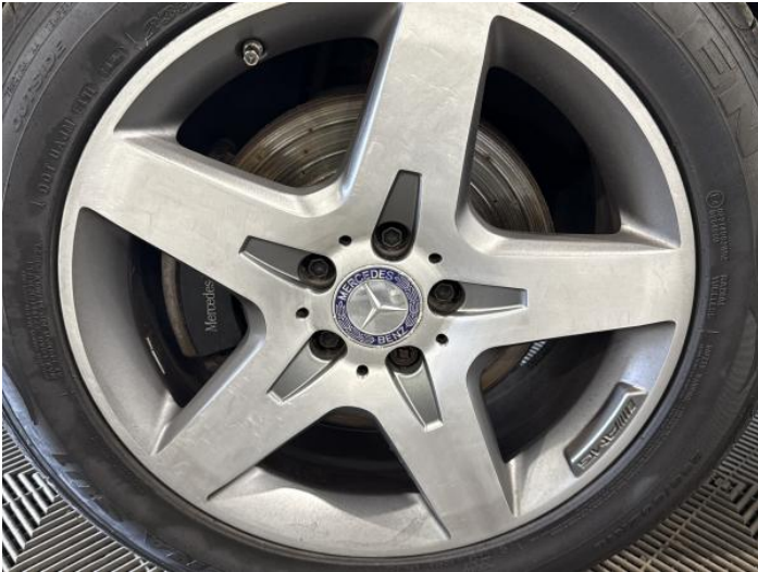
3: Wheel nsf Scratched Over 50mm
