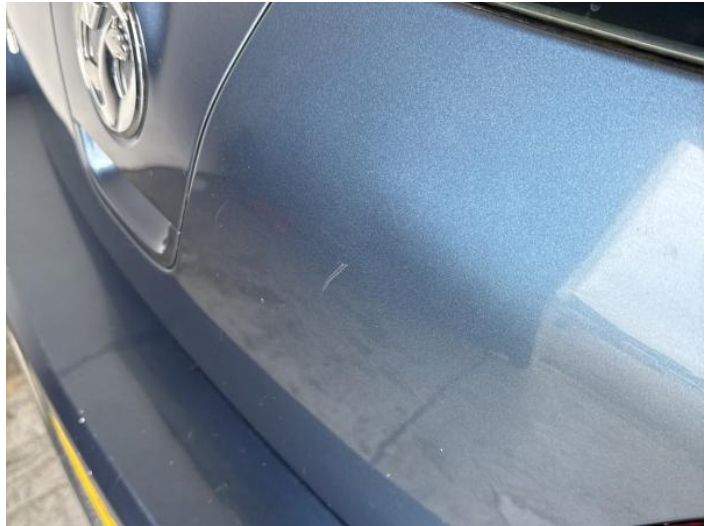
10: Tailgate Dented With Paint Damage
