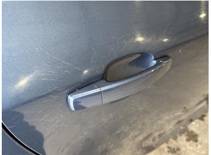
16: Door osr Scratched Over 25mm Thru Paint
