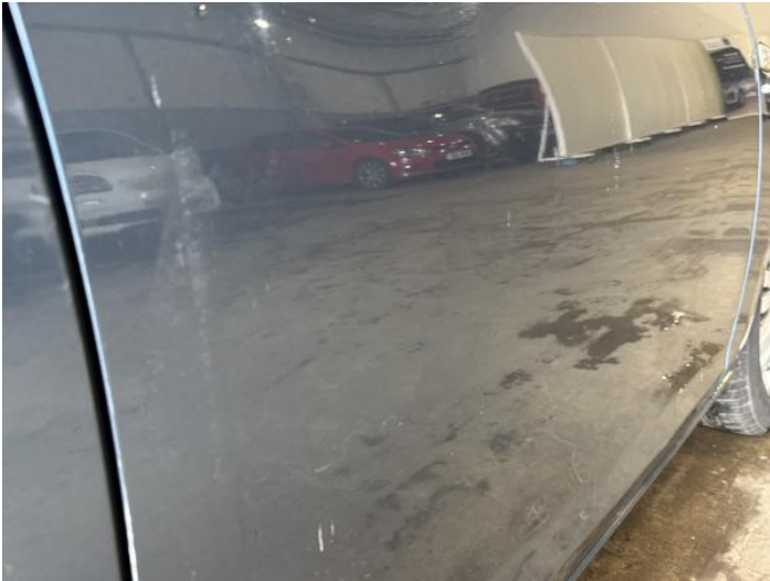
15: Door osf Dented With Paint Damage
