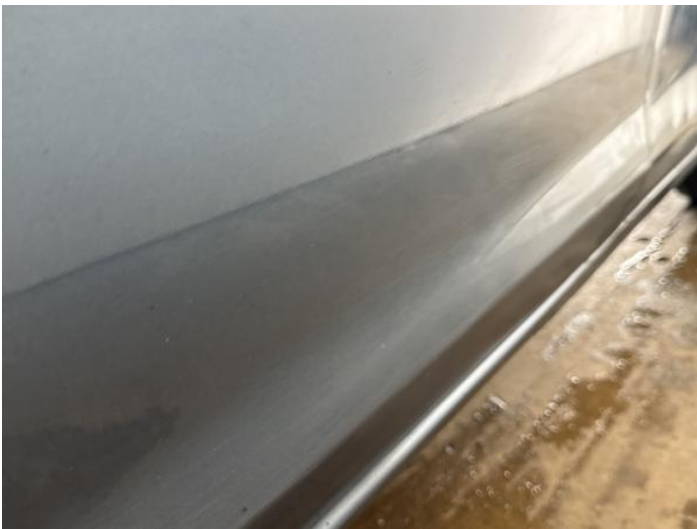
5: Door nsf Dented With Paint Damage
