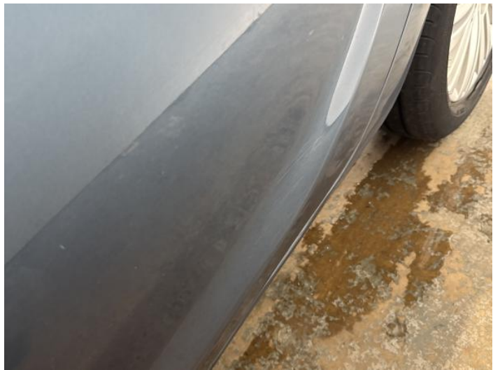
6: Door nsr Scratched Over 25mm Thru Paint
