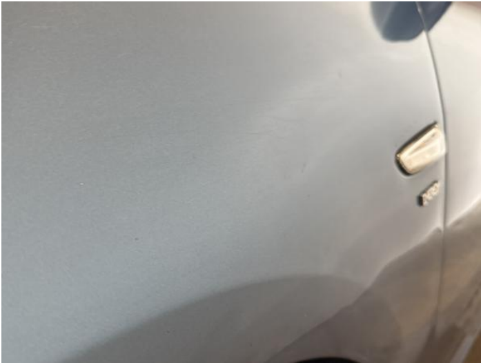
3: Wing nsf Poor Previous Repair Poor Paint
