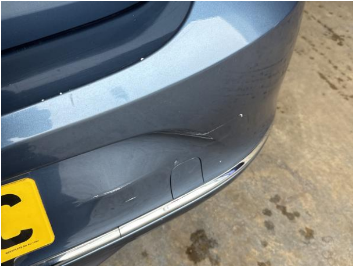
9: Bumper Rear Dented With Paint Damage
