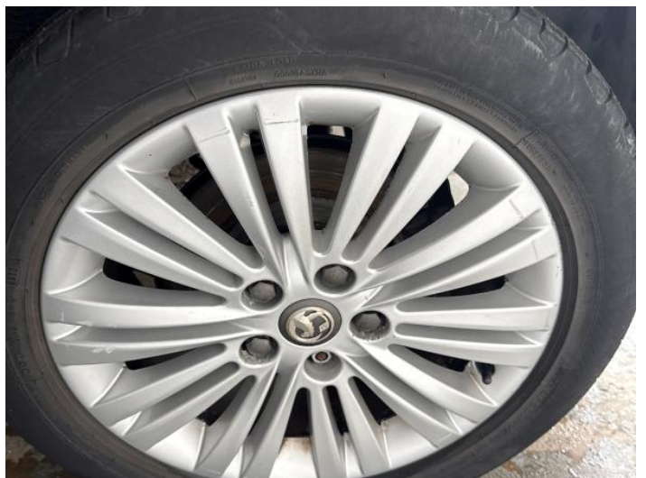
8: Wheel nsr Scratched Up To 50mm
