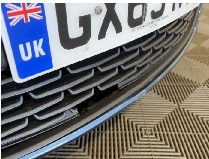
19: Bumper Front Grill Broken Replace
