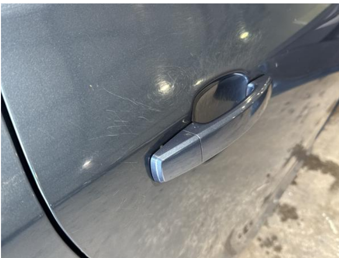
13: Door osr Scratched Over 25mm Thru Paint
