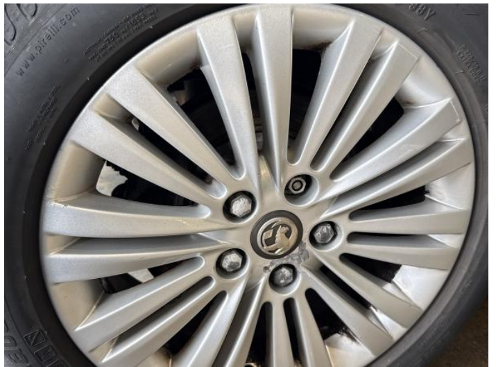
12: Wheel osr Scratched Over 50mm
