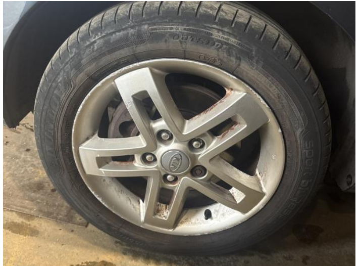
4: Wheel nsf Scratched Over 50mm
