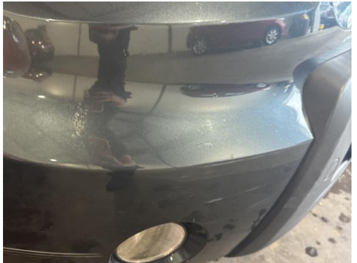
2: Bumper Front Scratched Over 100mm Thru Paint
