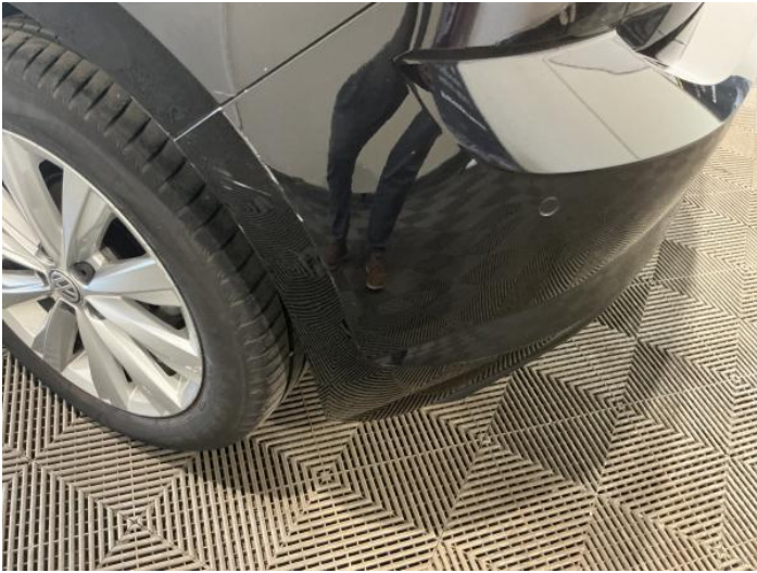
9: Bumper Rear Scratched 25 to 100mm Thru Paint
