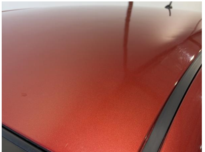
6: Roof Dented Hail - Severe
