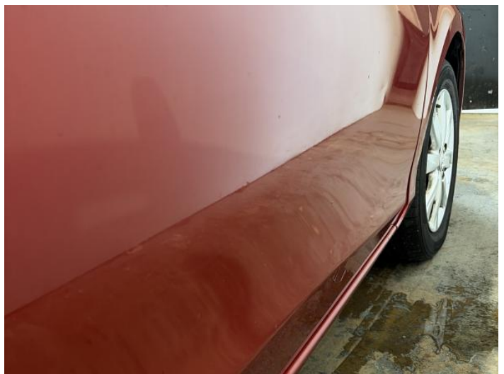
14: Door osf Dented Over 30mm
