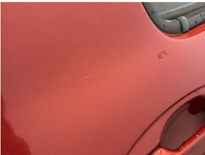
13: Door osr Scratched UpTo 25mm Thru Paint
