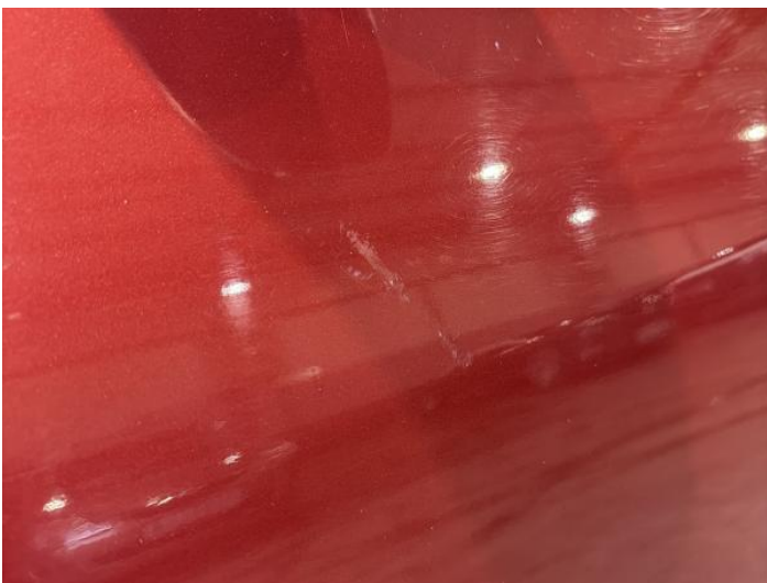
7: Door nsf Scratched Over 25mm Thru Paint
