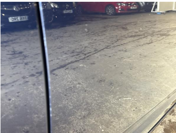
7: Door osf Scratched UpTo 25mm Thru Paint
