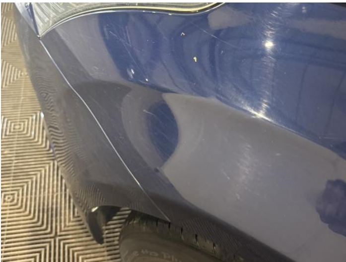
17: Wing nsf Scratched Over 25mm Thru Paint
