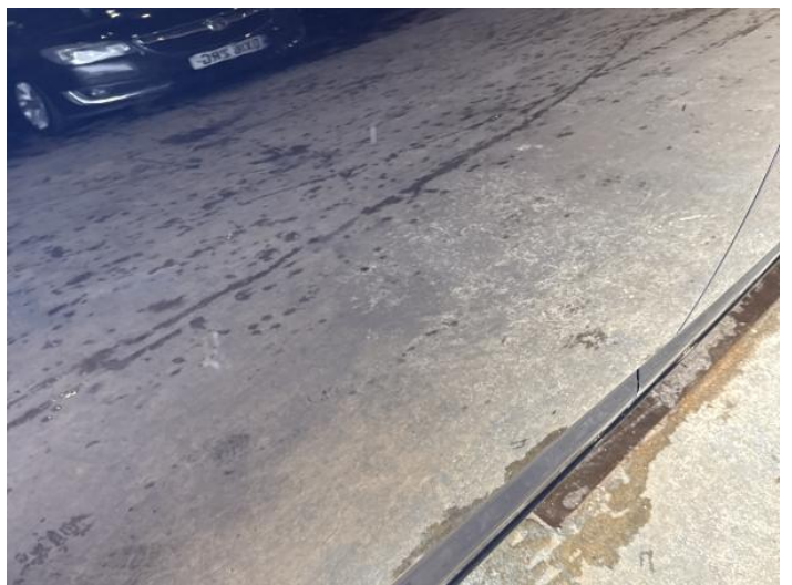
8: Door osr Scratched Over 25mm Thru Paint
