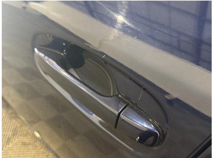
16: Door nsf Scratched UpTo 25mm Thru Paint
