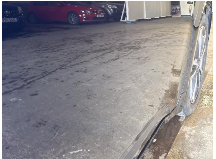
6: Door osf Dented Over 30mm
