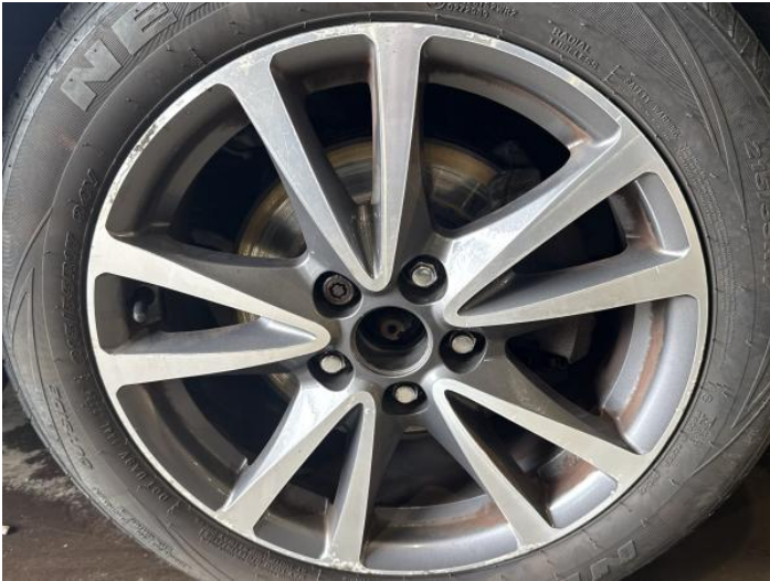
3: Wheel osf Scratched Over 50mm
