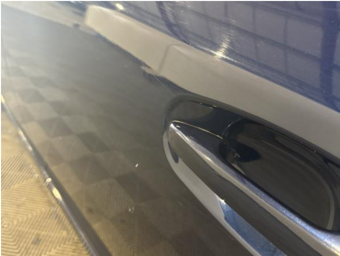
15: Door nsr Scratched Over 25mm Thru Paint
