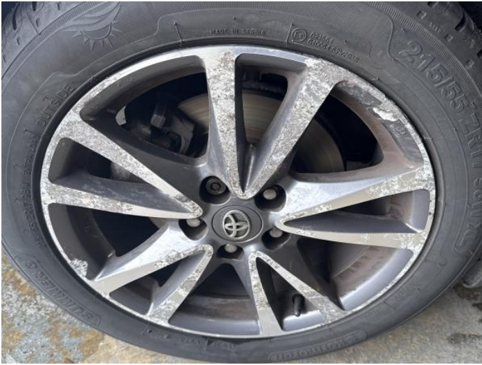
9: Wheel osr Scratched Over 50mm
