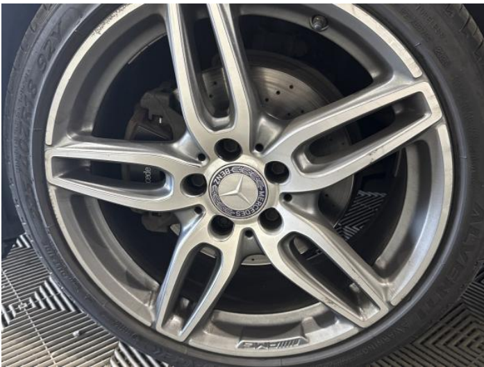
5: Wheel nsf Scratched Over 50mm
