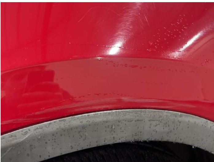
7: Wing nsf Scratched Over 25mm Thru Paint
