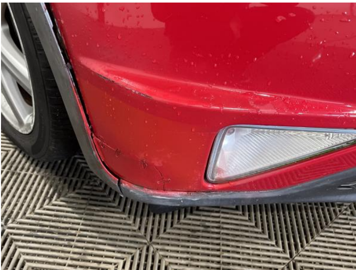
5: Bumper Front Cracked Over 25mm
