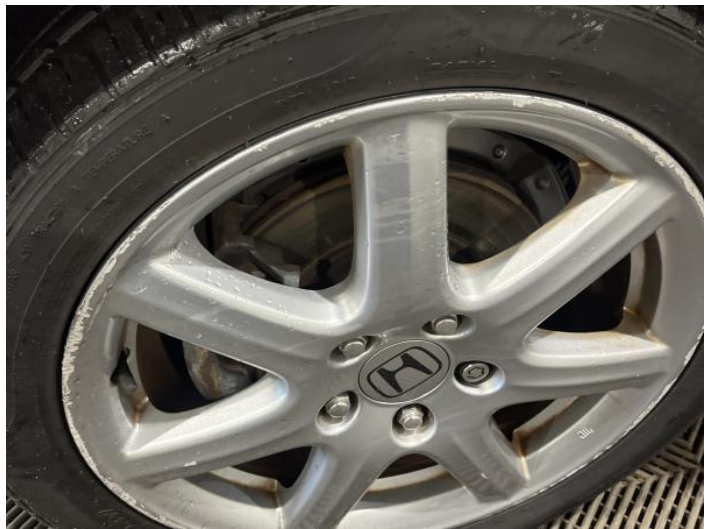
6: Wheel nsf Scratched Over 50mm
