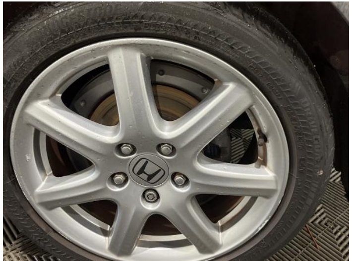
18: Wheel nsr Scratched Over 50mm
