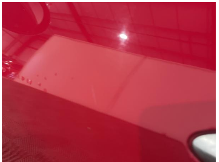
8: Door nsf Scratched Over 25mm Thru Paint
