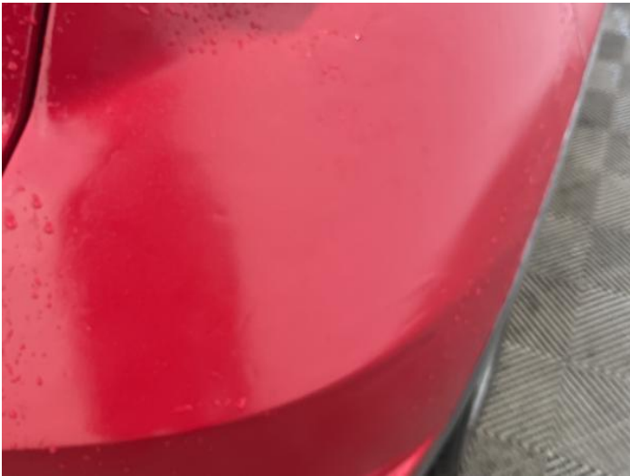
11: Bumper Rear Poor Previous Repair Poor Paint
