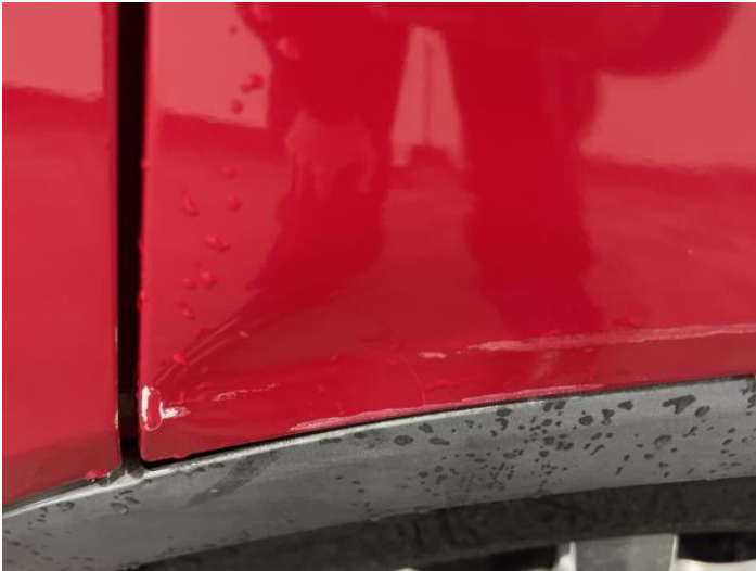
9: Qtr Panel nsr Dented With Paint Damage
