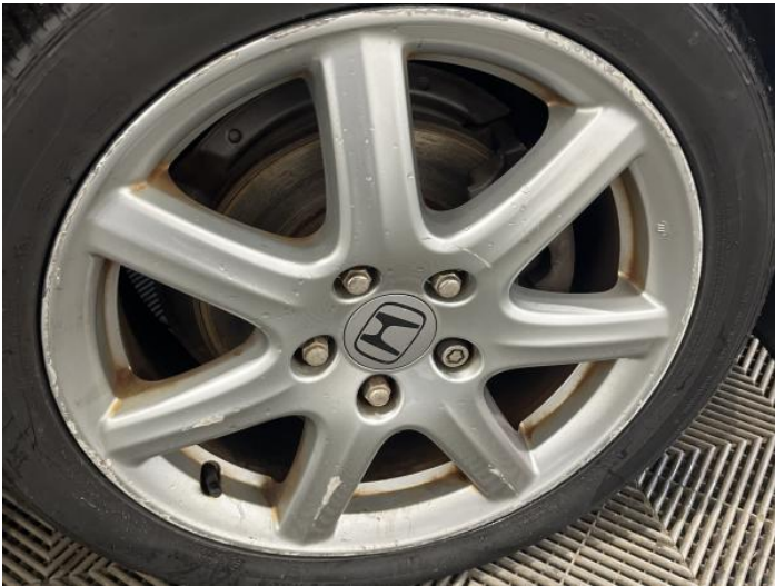
17: Wheel osf Scratched Over 50mm
