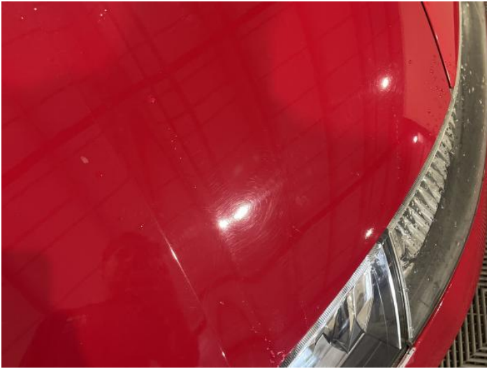
3: Bonnet Poor Previous Repair Poor Paint
