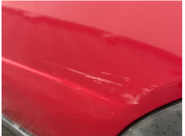
10: Door nsr Scratched Over 25mm Thru Paint
