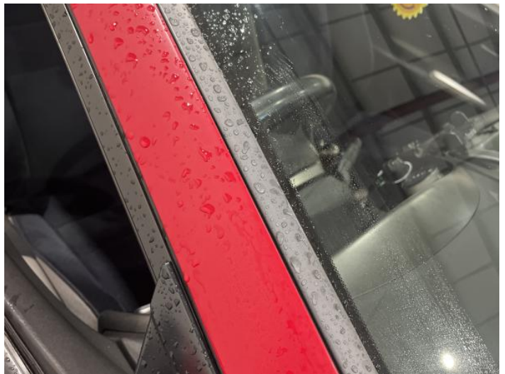
2: A Post os Poor Previous Repair Poor Colour
