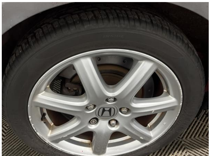
14: Wheel osr Scratched Over 50mm
