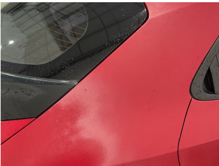
13: Qtr Panel osr Poor Previous Repair Poor Paint
