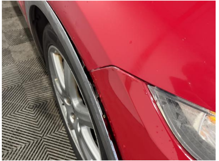
4: Wheel Trim nsf Broken Replace
