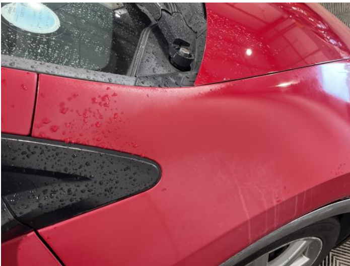
1: Wing osf Poor Previous Repair Poor Paint
