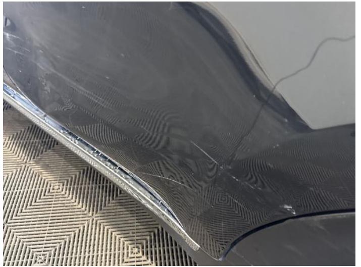
6: Door nsr Dented With Paint Damage
