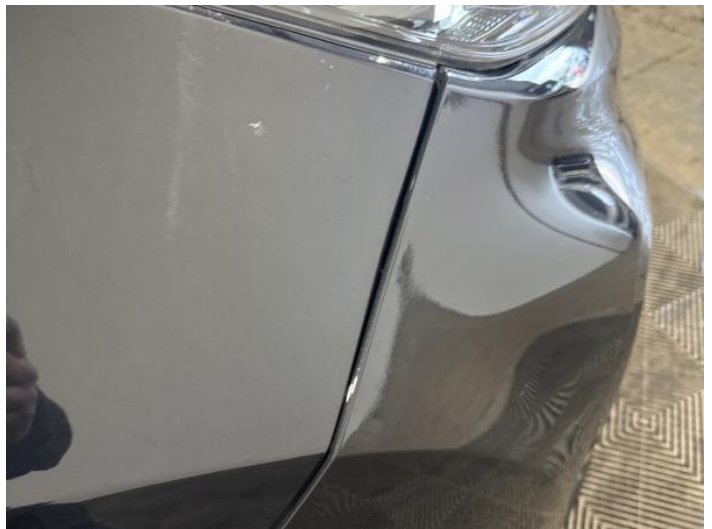
18: Bumper Front Insecure Action Required
