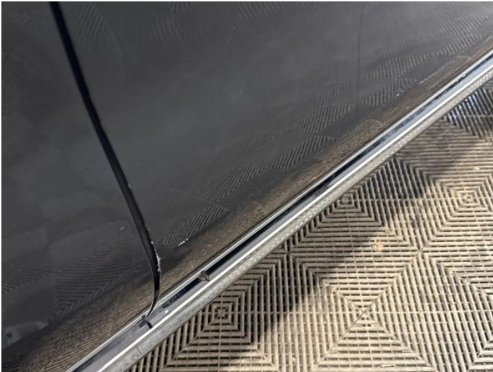
15: Door osf Scratched Over 25mm Thru Paint
