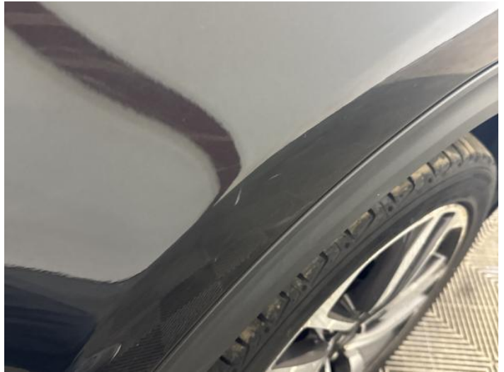
16: Wing osf Scratched UpTo 25mm Thru Paint
