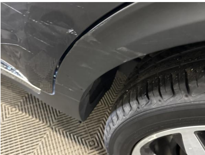
7: Qtr Panel Arch Extension ns Scuffed (Unpainted) Over 100mm
