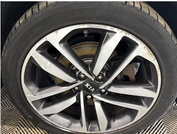
17: Wheel osf Scratched Over 50mm
