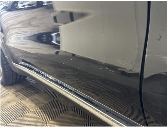
5: Door nsf Scratched Over 25mm Thru Paint
