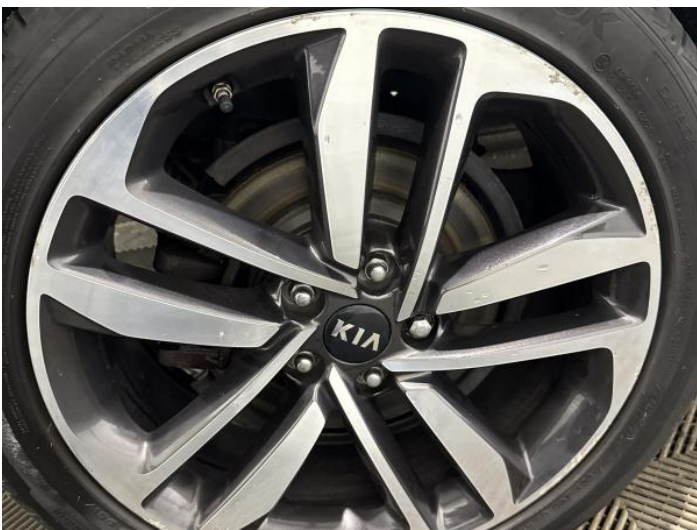
13: Wheel osr Scratched Over 50mm
