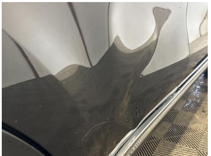
14: Door osr Dented Over 30% Of Panel
