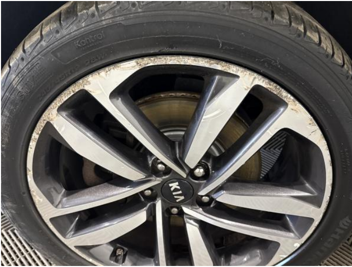
3: Wheel nsf Scratched Over 50mm
