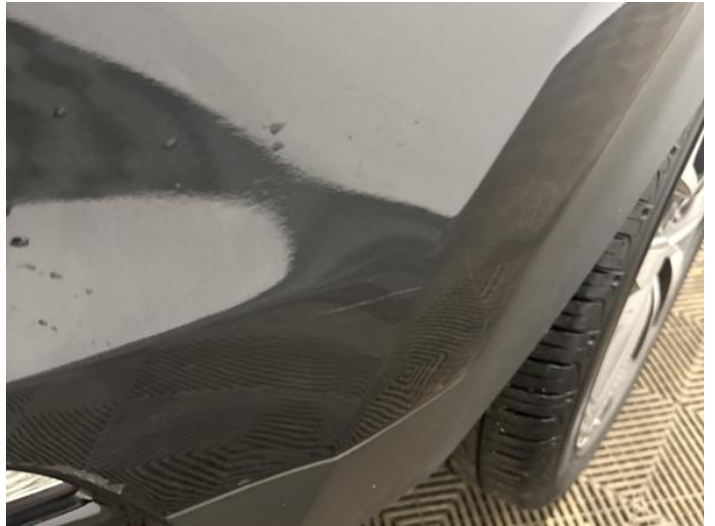
10: Bumper Front Scratched 25 to 100mm Thru Paint
