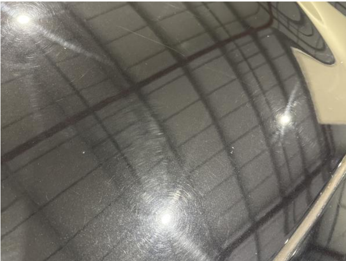
1: Bonnet Scratched Over 25mm Thru Paint
