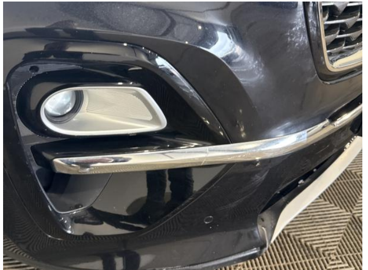
2: Bumper Front Scratched 25 to 100mm Thru Paint
