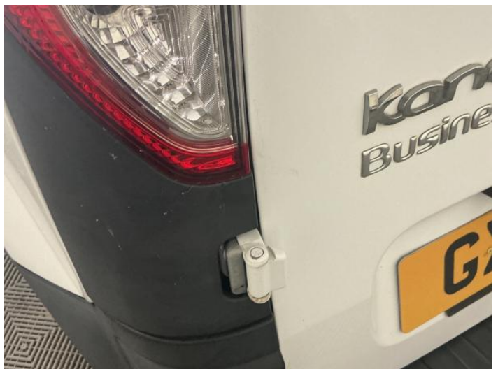
8: Bumper Rear Moulding Scuffed (Unpainted) Over 100mm
