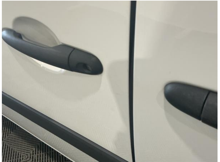
4: Door nsf Dented Over 2 UpTo 10mm
