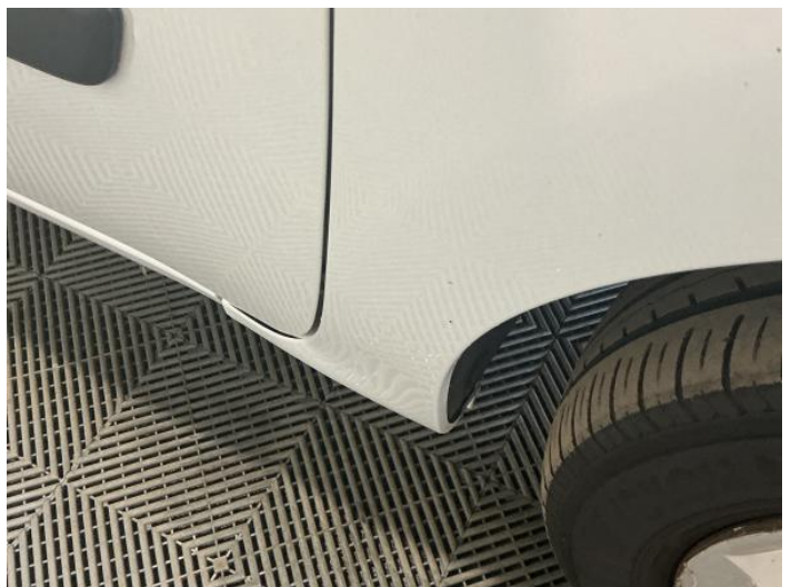
14: Wing osf Dented Over 30mm
