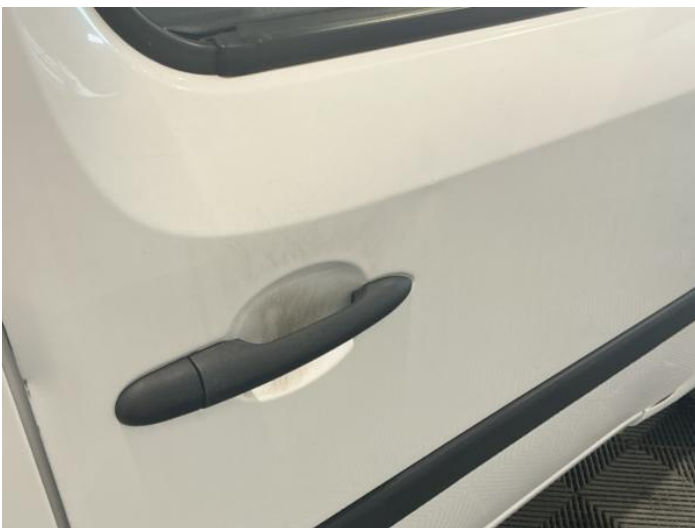
13: Door osf Dented With Paint Damage
