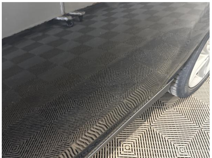
8: Door nsr Dented Between 10mm + 30mm
