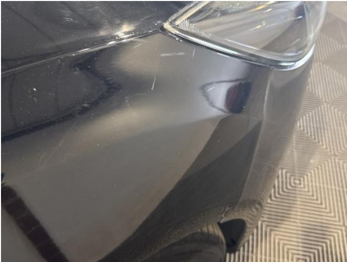
21: Wing osf Scratched Over 25mm Thru Paint
