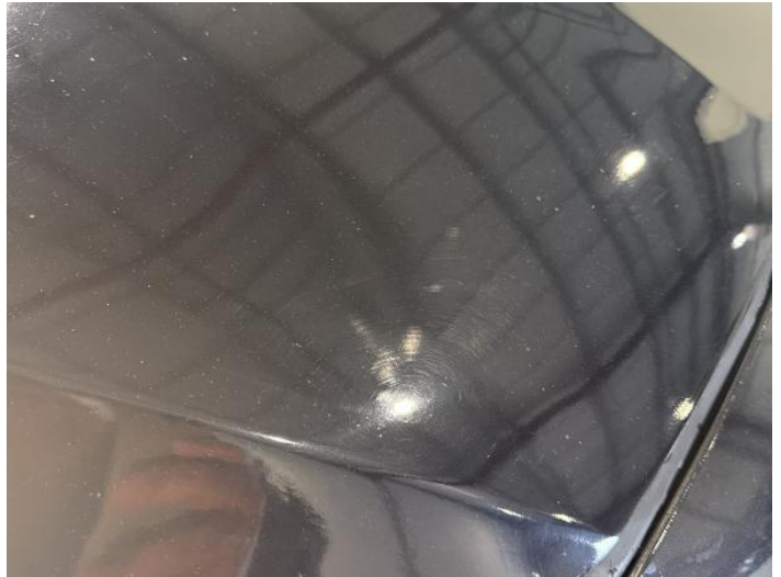
4: Bonnet Poor Previous Repair Poor Paint
