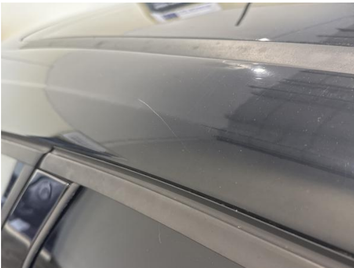
23: B Post os Scratched Over 25mm Thru Paint
