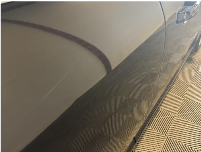
17: Door osr Dented Between 10mm + 30mm
