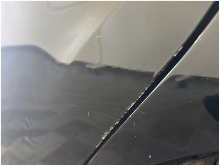
9: Door nsr Chipped Edge Chip
