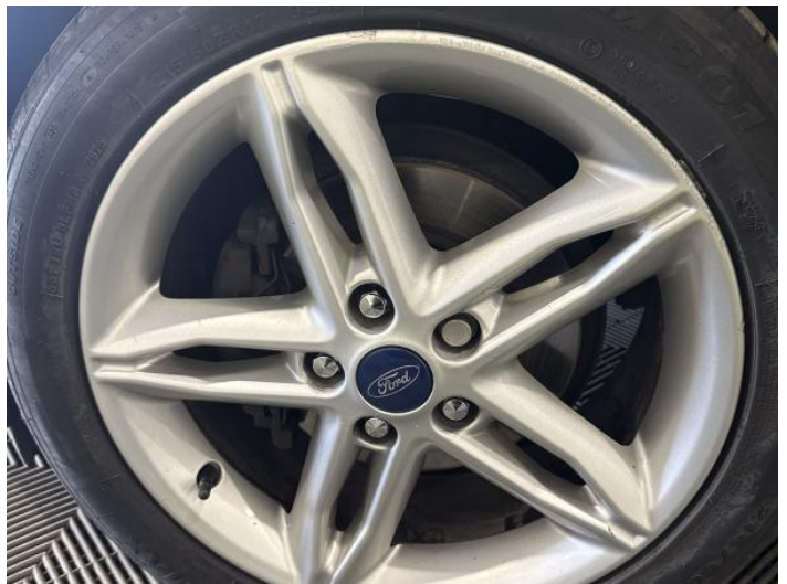
6: Wheel nsf Scratched Over 50mm
