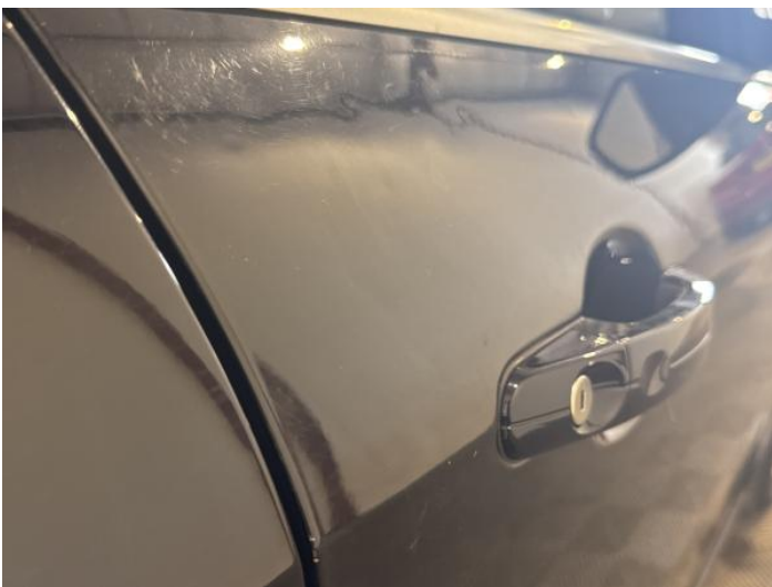
19: Door osf Dented Over 30mm
