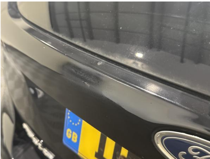
11: Tailgate Poor Previous Repair Poor Paint
