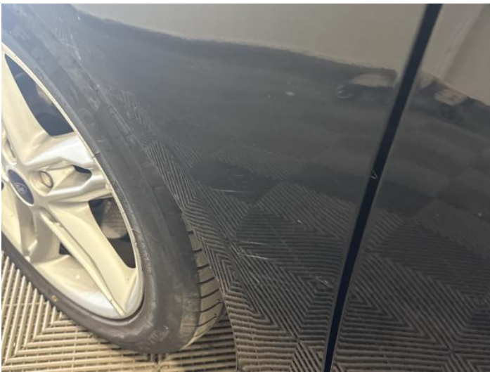
5: Wing nsf Scratched Over 25mm Thru Paint
