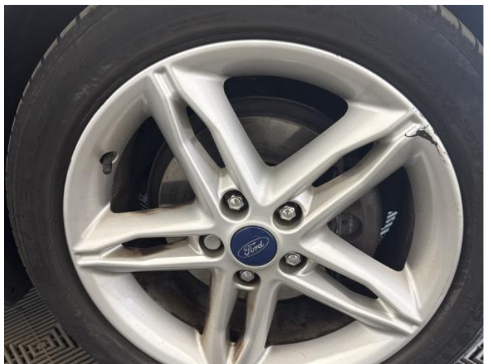
20: Wheel osf Scratched Over 50mm
