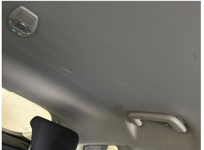
2: Roof Lining Scuffed Over 25mm
