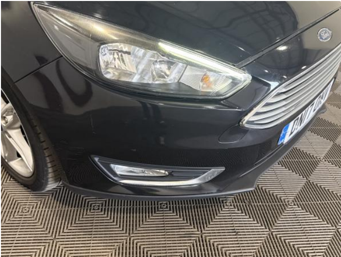
3: Bumper Front Poor Previous Repair Poor Paint
