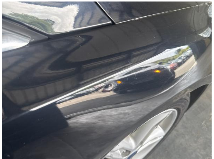
24: Wing osf Dented Between 10mm + 30mm
