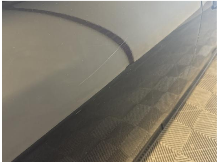
16: Door osr Scratched Over 25mm Thru Paint
