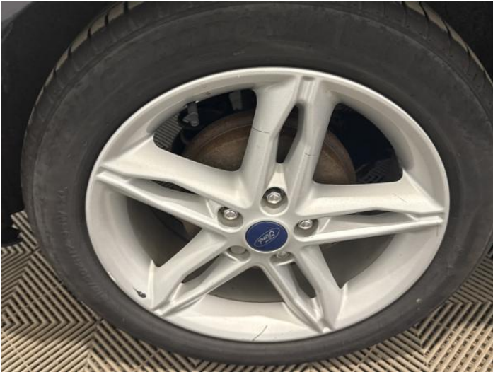
15: Wheel osr Scratched Over 50mm
