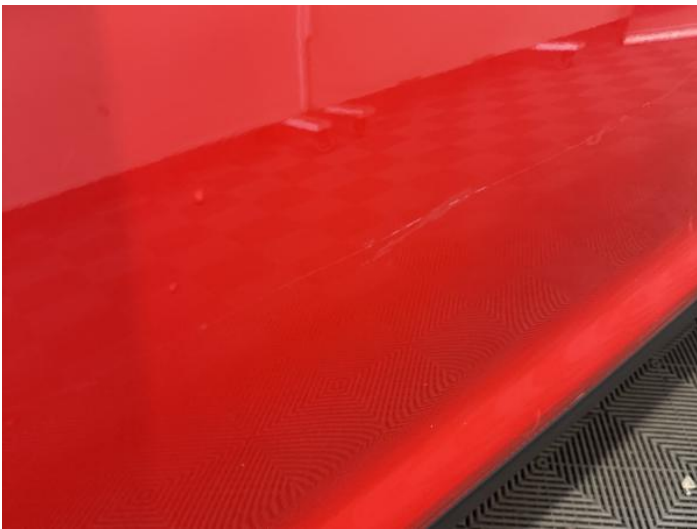
5: Door nsf Scratched Over 25mm Thru Paint
